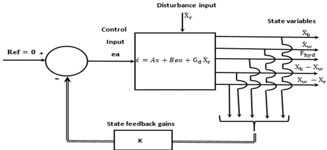
Fig. 8 Full-state feedback control applied to state-space model.
