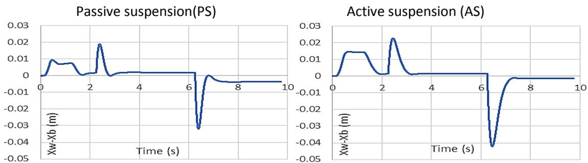
Fig. 17 The suspension movement for PS and AS.
