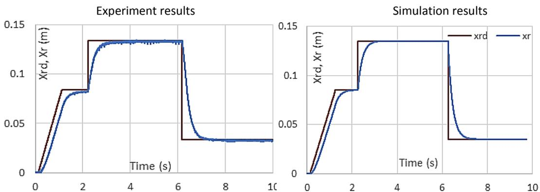
Fig. 11 Comparison of the desired and measured step input  $X_{rd}$ ,  $X_r$  (m) (1).
