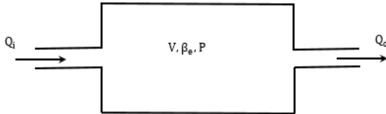
Fig. 6 Flows entering and leaving a control volume.
