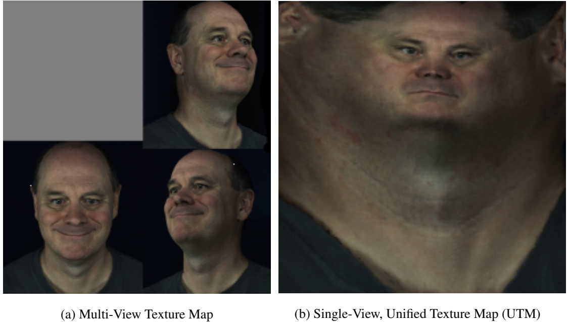
Figure 3.13: The figure shows (a) multi-view texture map and (b) unified texture map.
