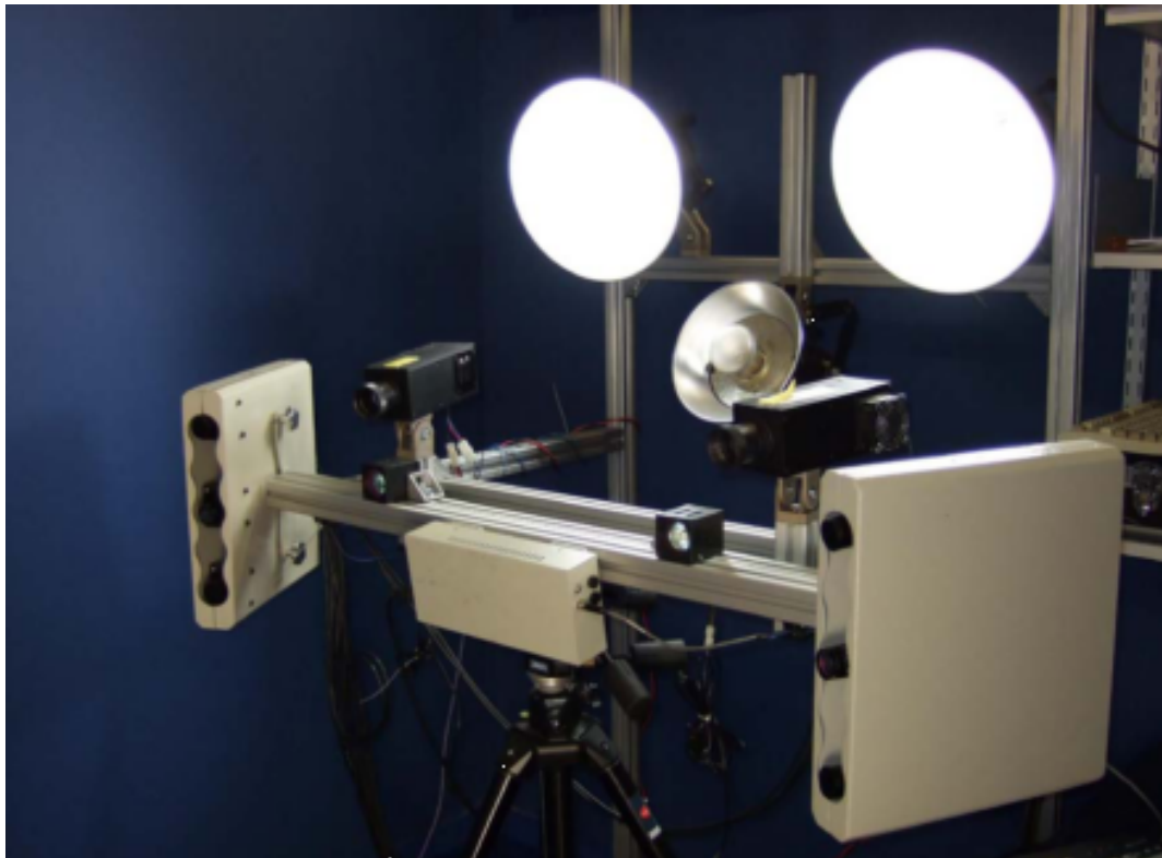
Figure 3.1: Figure shows the old generation of 3dMD capture system used to capture the 3D data for our research over the first four years employing two pods system comprising of six cameras; two colour and four grey scale.
