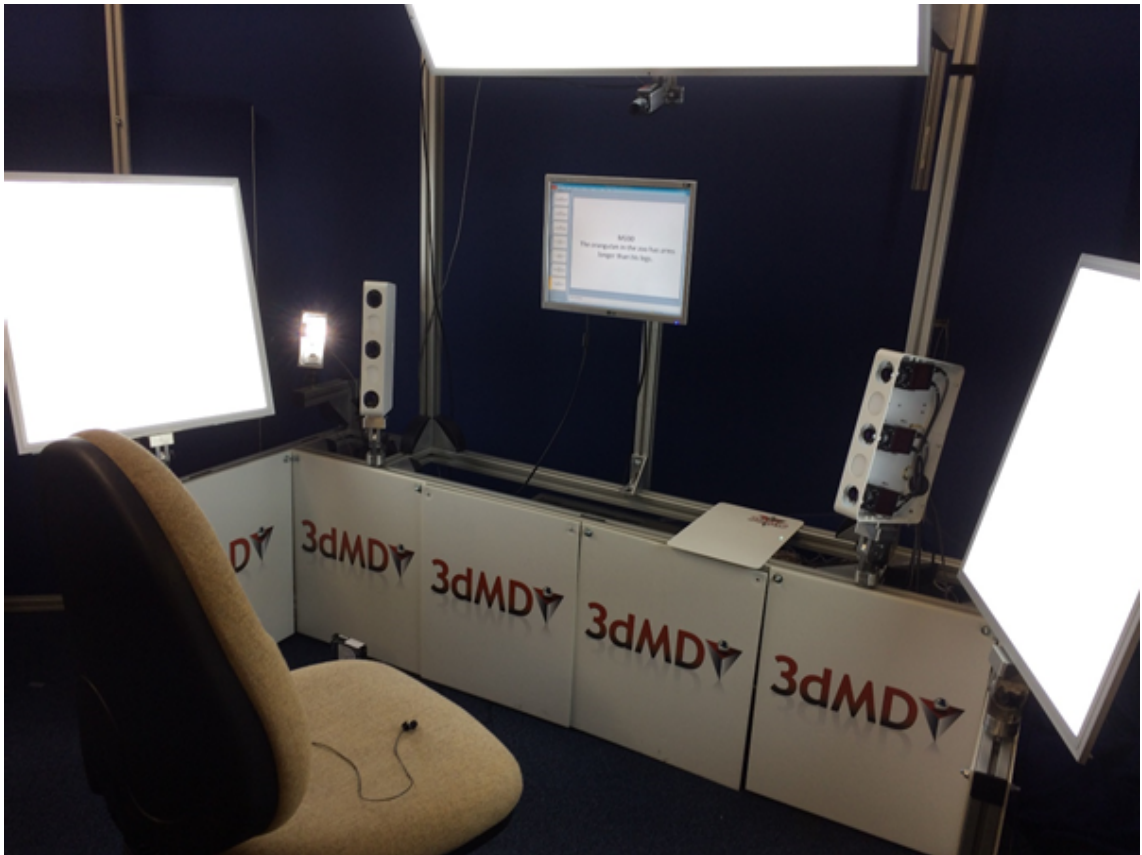
Figure 3.4: Figure shows the last generation of 3dMD capture system used to capture the remaining data for our research over the last five years, consisted of two pods containing two mono cameras on the top and bottom, with a colour camera in the middle.
