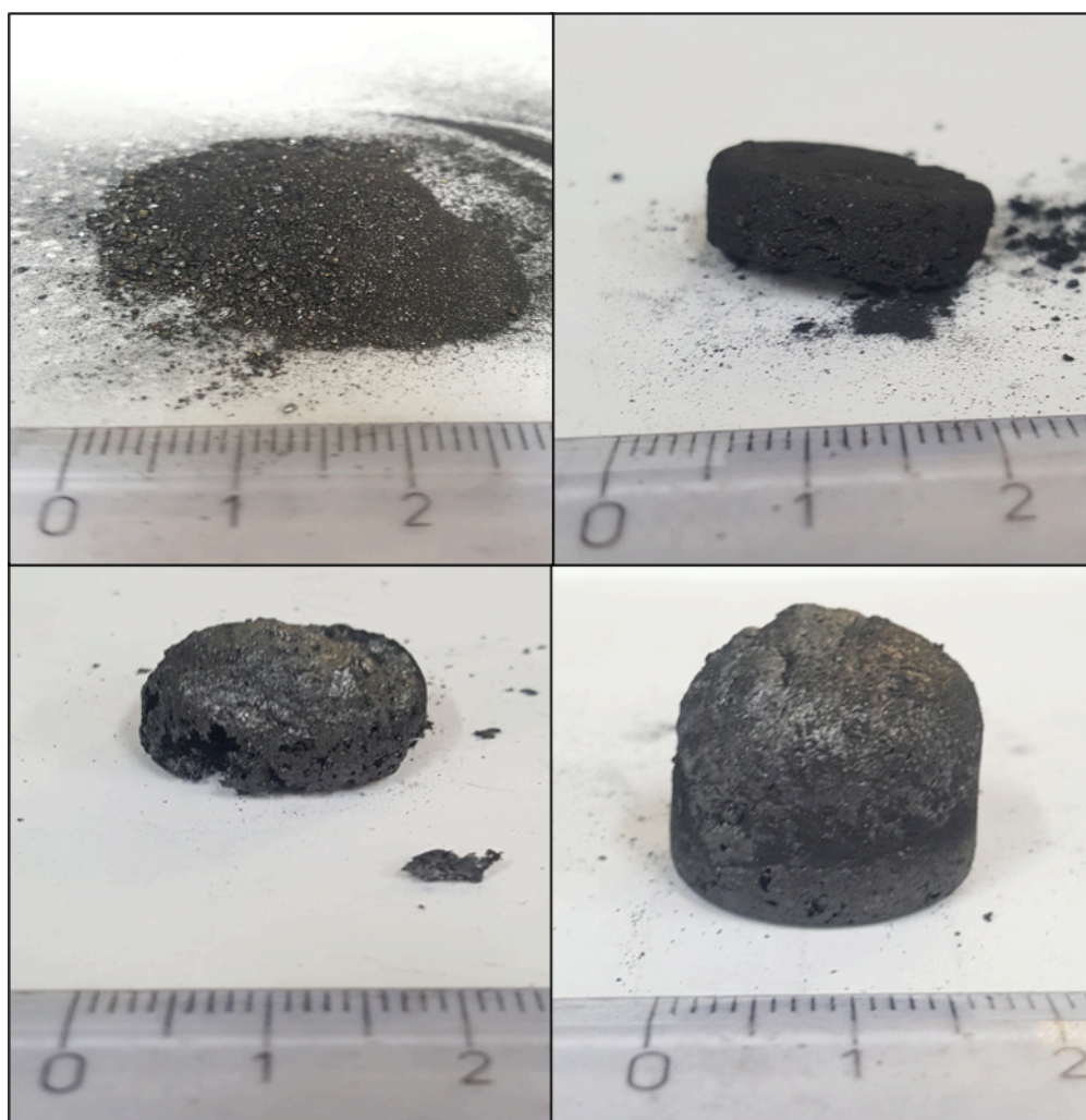
Figure 19: Agglomeration Index residues by which caking scores are determined. Clockwise from top left: LV1 residue, MV3 residue, MV4 residue, HV1 residue
