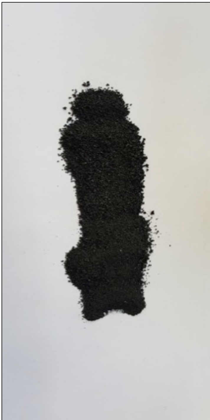
Figure A 1: Post DTF non-agglomerated char sample (MV3) remaining as powder
