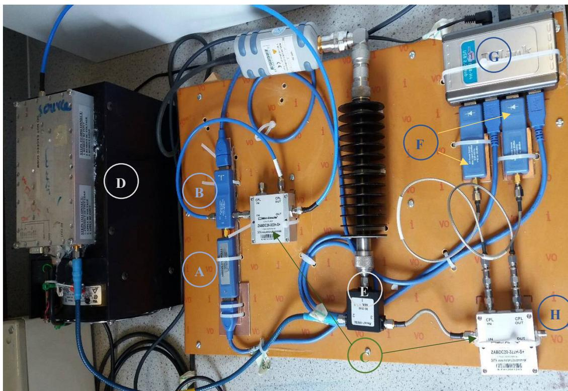
The microwave system used in this project. A: signal generator. B: RF switch. C: bi-directional couplers. D: Power amplifier. E: Circulator. F: power sensors. G: Controller. H: connection to the microwave cavity.
