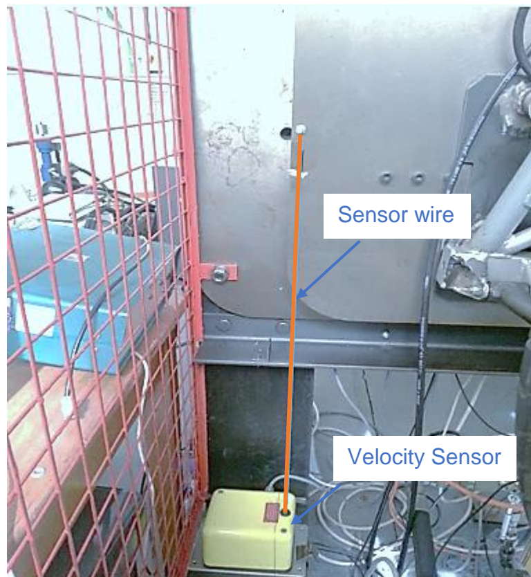
Fig. 2.22. Photograph of the installation of the velocity sensor for the measurement of car body velocity and displacement.
