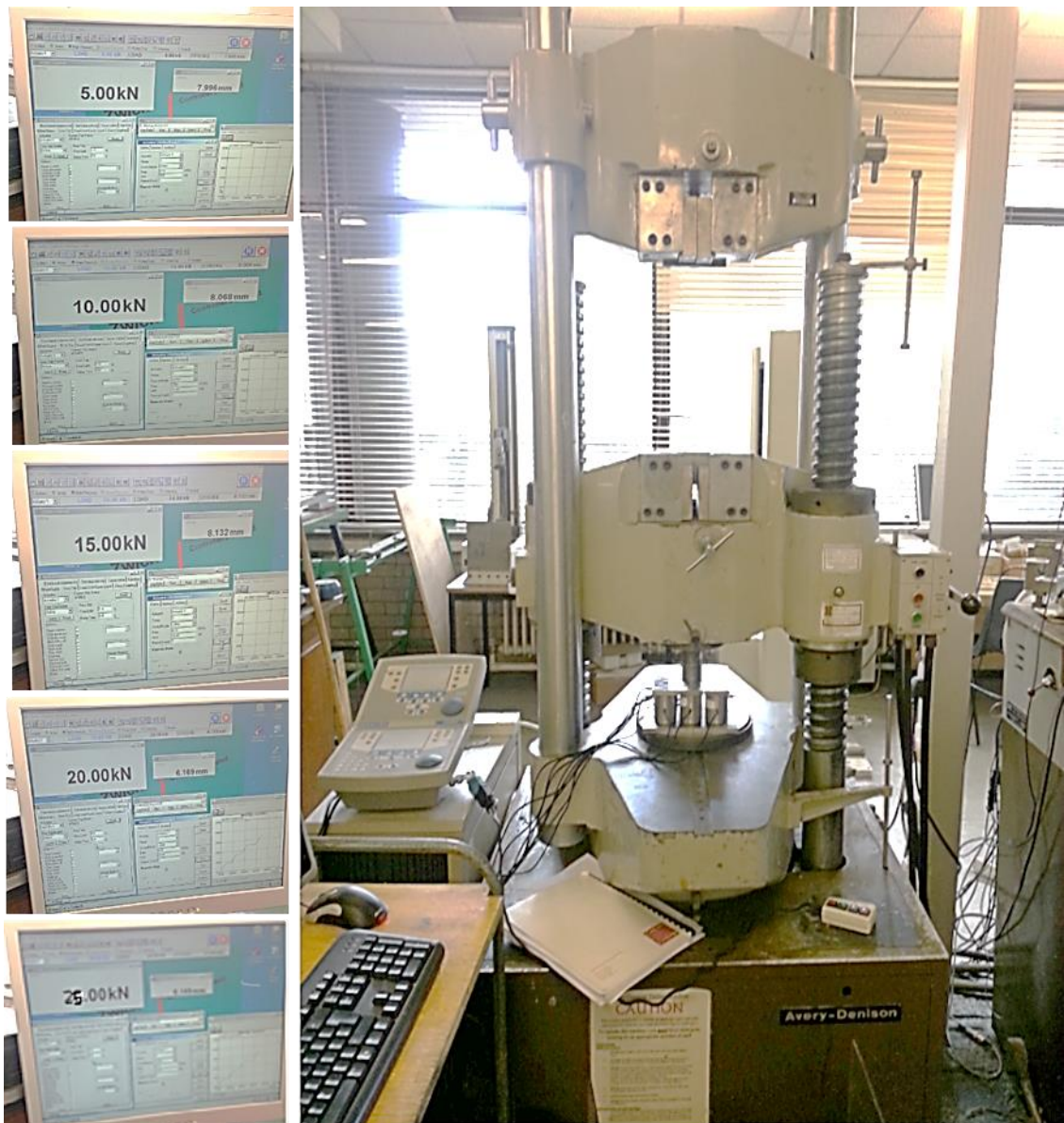
Fig 2.19. Test rig used for the calibration of the load cells.
