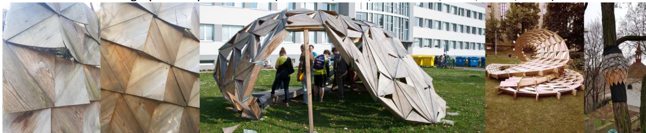
Figure 4: Different life stages after extensive weathering of wood responsive prototypes from left to right: a responsive screens Ray 2 after five years and a Ray 3 after three years, both inhabited by algae, lichen and blue stain fungus (the Ray 3 screen has washed out sugar by salt for preventing an interaction with decaying species); responsive pavilion pareSITE after one and half year of struggling with the interaction of torqued forces within the geometrical structure of Möbius strip with weather extremes of two summers and one winter; a collapse of the LOOP responsive wooden pavilion after the gardener ignored the requirement of turning of the sprinklers that watered the sunny oriented half of it in arid season (the pavilion was afterwards rebuilt at different location) ; and a responsive insect hotel TreeHugger CZ after one and half year fully co-performing with surrounding eco-system, being inhabited by both insects and algae. The prototypes were built within the framework of Collaborative Collective, Defio, s.r.o., Oximoron, Re.Code.Nature, ARCHWERK, Architectural Institute Prague, FA TUL, FLD CZU and CoolAND (photos: Davidová and Novotná 2014-2018)
