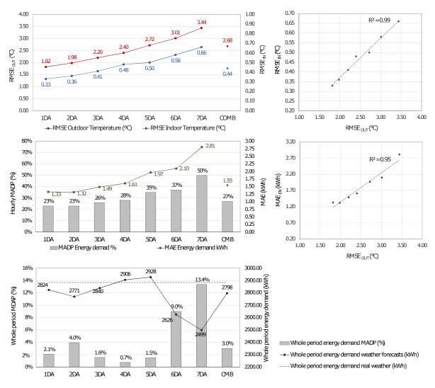
**Figure 9.** (**above**): comparison between hourly outdoor temperature error (*RMSE*) and hourly mean indoor temperature error (*RMSE*) for the different day-ahead forecasts. (**middle**): *MAE* and *MADP* for hourly energy demand for the different day-ahead forecasts. (**below**): *MADP* and energy demand for the whole period of study for real weather and forecast weathers
