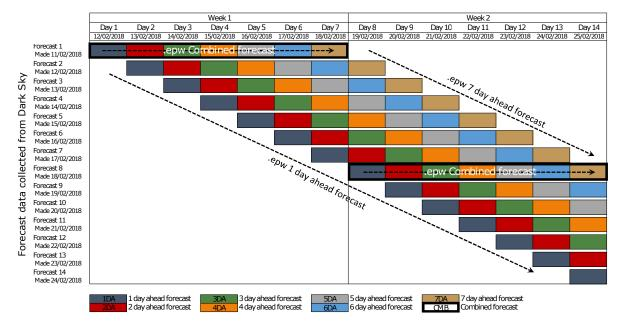
Figure 4. Organization of forecast data and construction of forecast weather files.
