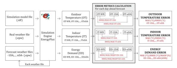
Figure 8. Building energy model (BEM) simulation and error metrics calculation scheme.
