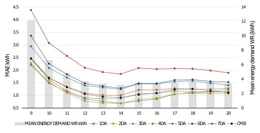
Figure 10. Error metric (MAE) for the energy demand hour-by-hour.
