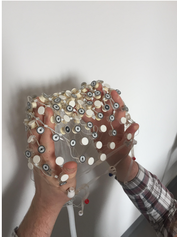
Figure 2-5. The 64-channel Hydrocel Geodesic Sensor Net (Electrical Geodesics, Inc.).
