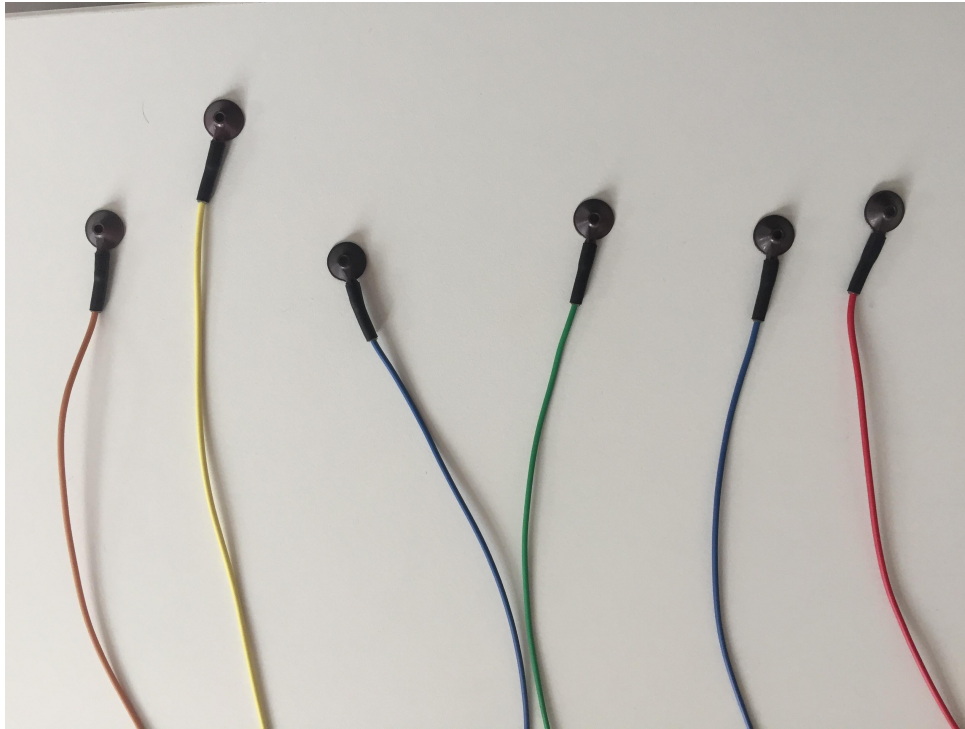
Figure 2-6. The silver-chloride electrodes, used in the EEG studies described in this thesis.
