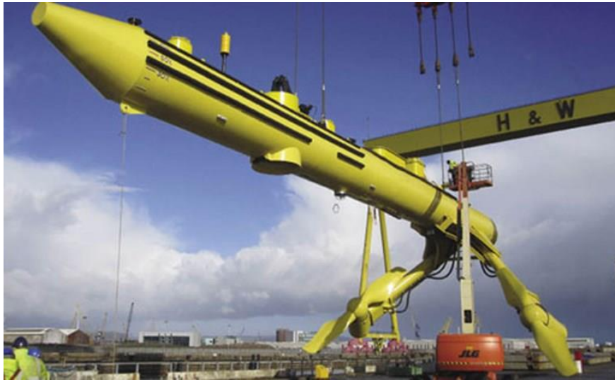
Figure 2-11 Scotrenewable turbine ready to be installed (Image Source: renews.biz)
