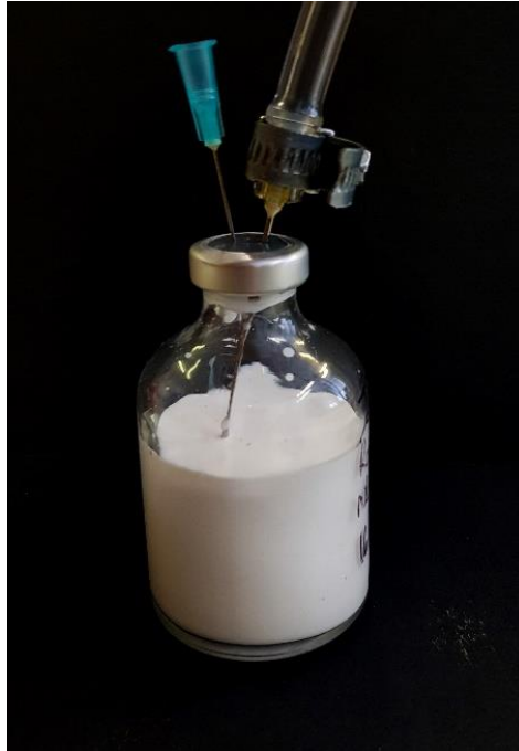
Figure 3.4 50 ml glass vial with 50 ml Lipid emulsion showing oxygen removal procedure through nitrogen flushing.
