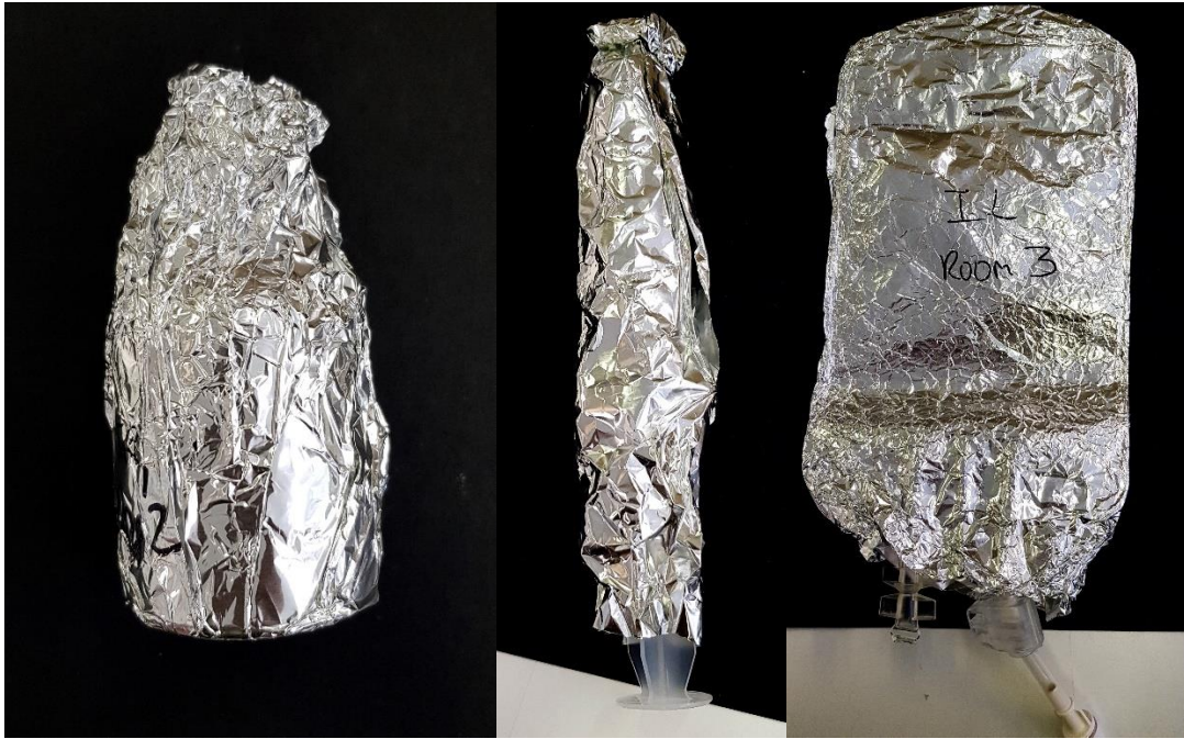
Figure 3.5 Light protected 50 ml glass vial, 50 ml syringe and 250 ml multi-layer PN bag covered with aluminium foil.
