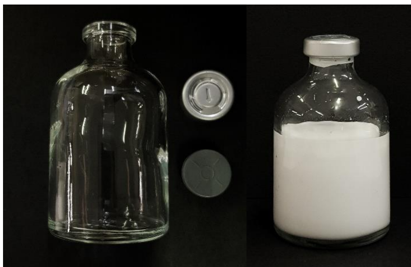
Figure 3.3 50 ml glass vial with rubber septum and metal clasp filled with 50 ml lipid emulsion.
