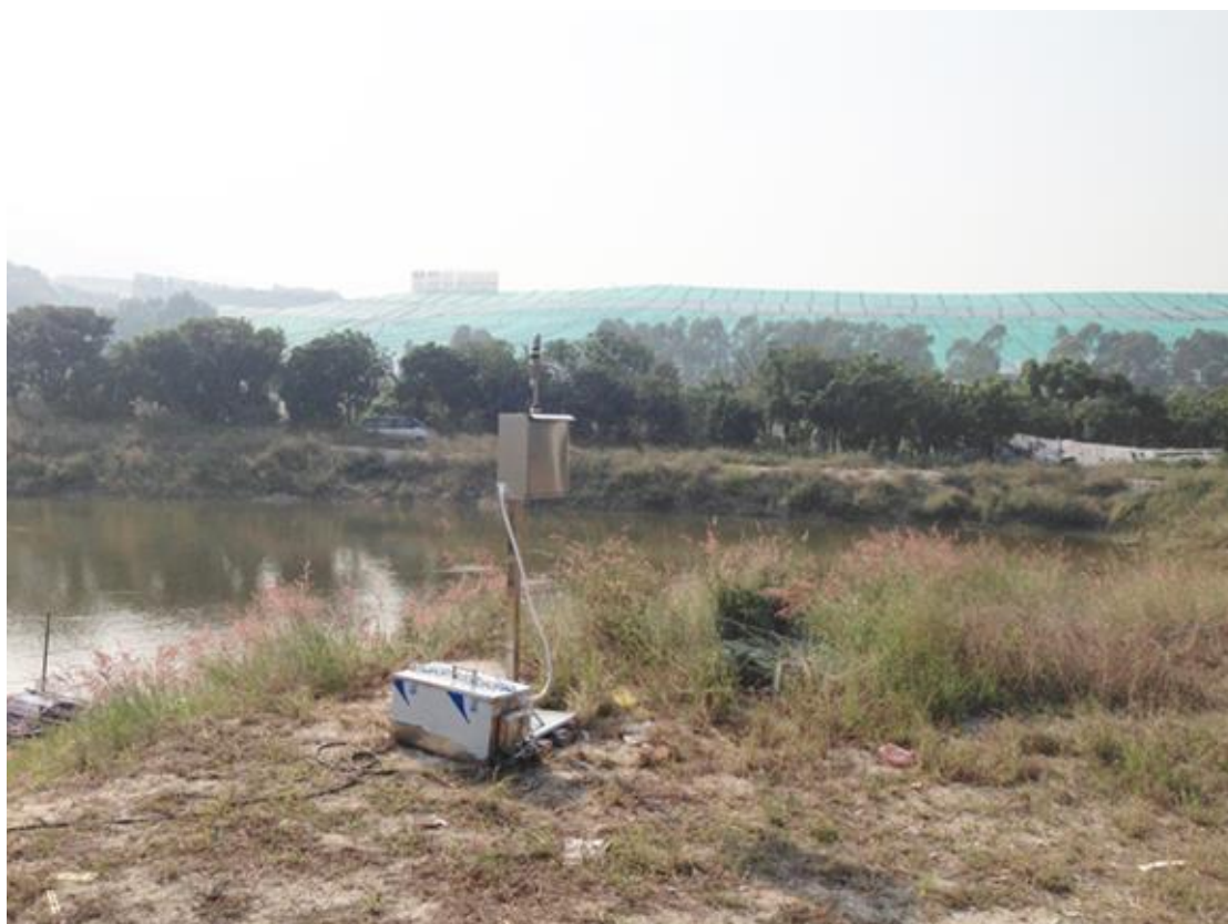
86 Figure S3 URG PM 2.5 filter-based sampler at WENT sampling location.
