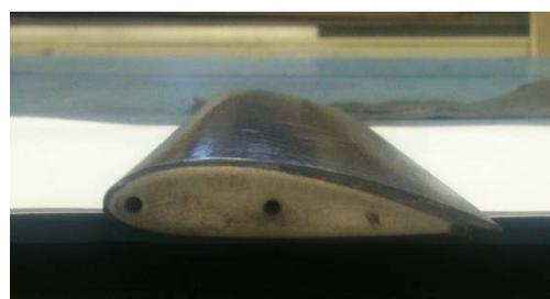
Figure G20. Blade after surface finishing
