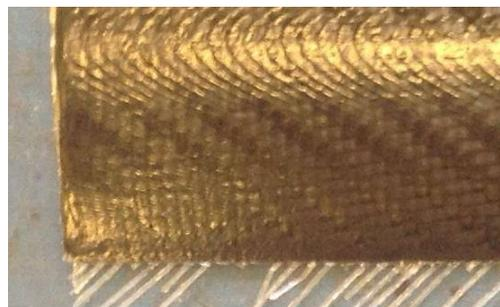
Figure G38. Very smooth surface with some hardened resin strings attached to it.
