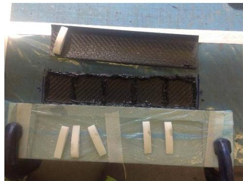
Figure G18. Assembling blade and inserts
