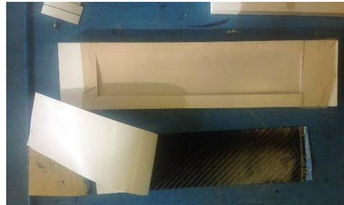
Figure G7. Cutting stripes of carbon fibre
