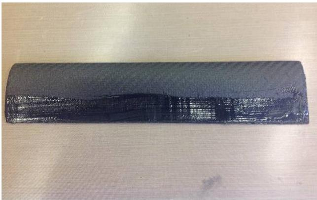
Figure G28. Grouted edge of the blade
