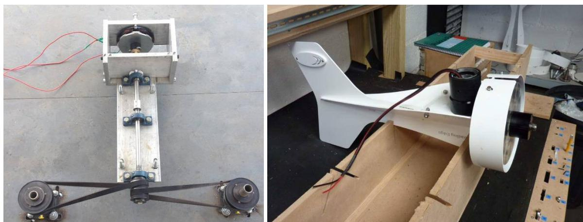
Figure H8. LHS, Generator built in VAT-PTO, RHS, generator built into a wind turbine housing [185]
