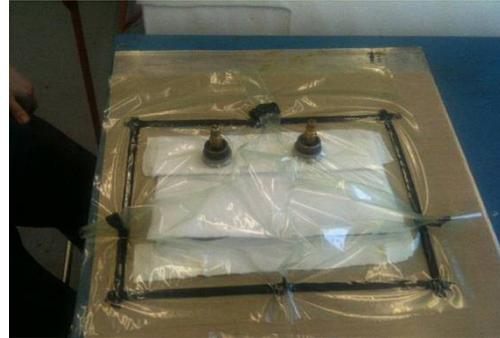
Figure G25. Vacuum bag attached to a metal sheet
