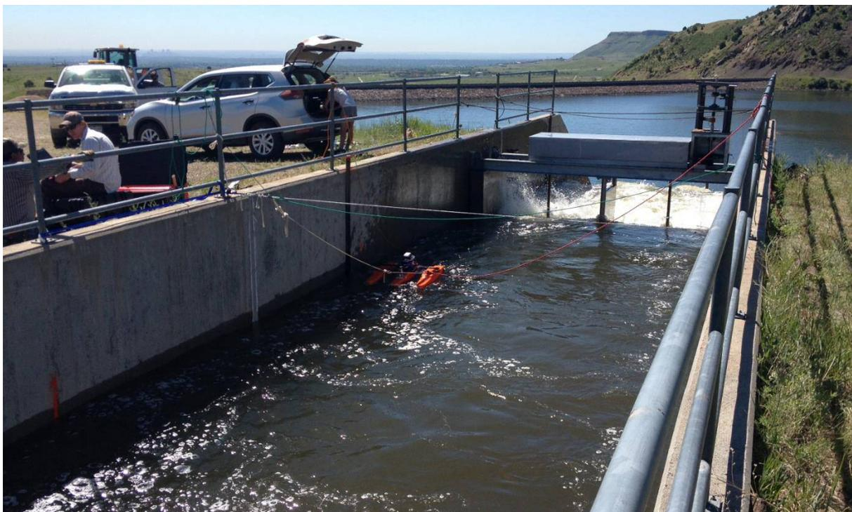
Figure F2. Velocity measurements taken by the US Bureau of Reclamation during testing [180]
