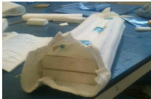
Figure G35. Setting-in stripes on the mould
