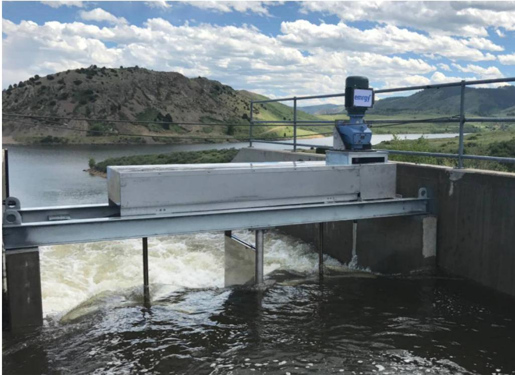
*Figure 102. Hydrokinetic twin VAT in full scale, installed in South Bolder Canal near Denver*
