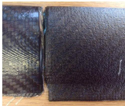
Figure G26. Left hand side (smooth), mould was used, right hand side (rough), no mould was used
