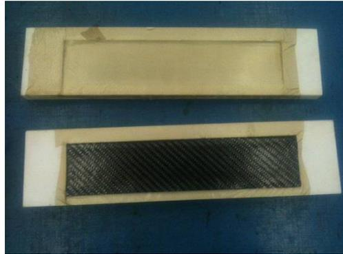
Figure G34. Wrapped core placed in the mould
