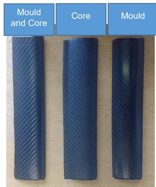
Figure G39. Finished blades in comparison
