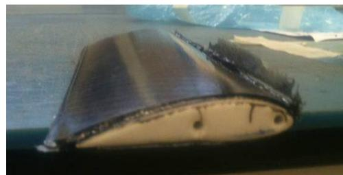
Figure G19. Assembled blade after gluing together
