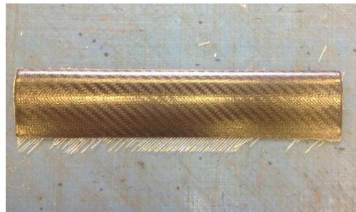
Figure G37. Released blade after curing
