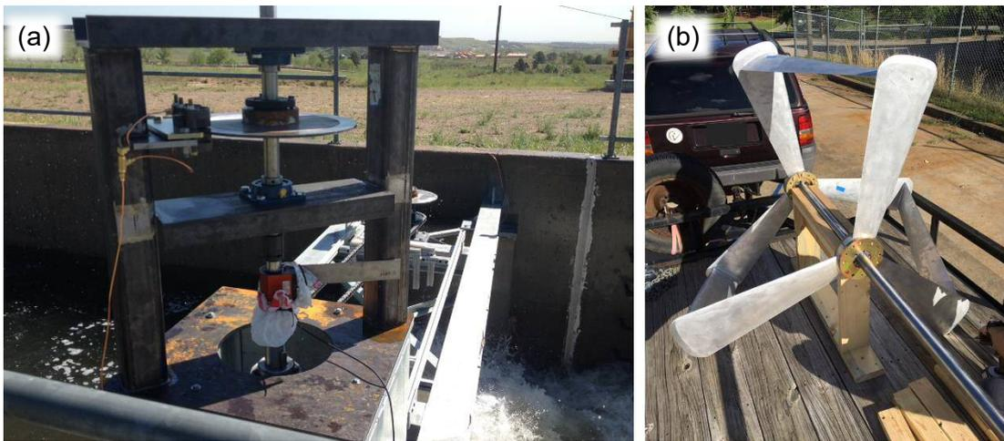
Figure 104. a) Mechanical PTO featuring hydraulic disc brake and torque transducer; b) VAT rotor prior to installation
