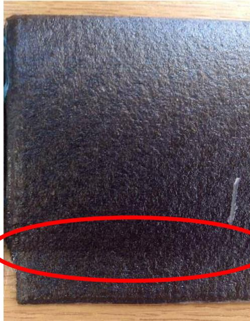
Figure G27. Buckled section of blade surface
