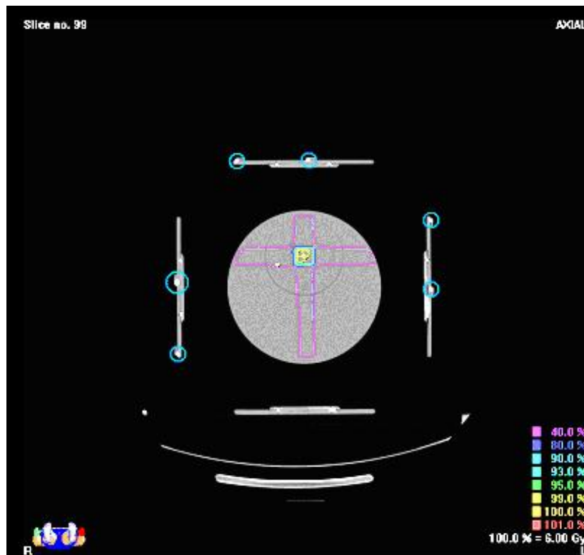
Figure 1.4: Stereotactic phantom scanned in the BrainLAB localiser box indicating position of localiser bars.
