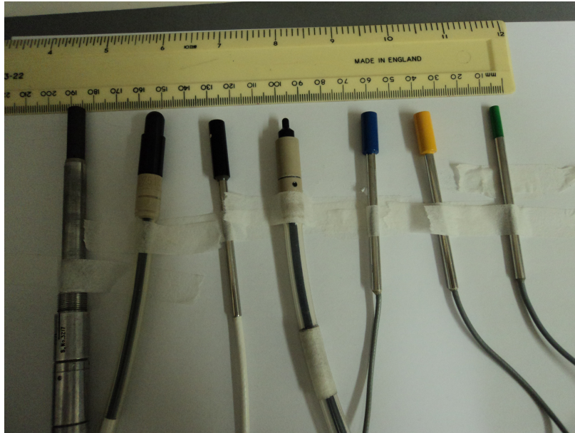
Figure 5.1: Photograph of detectors used in small field investigations. From left to right, Farmer, CC13, RK, CC01, EFD, PFD, SFD.
