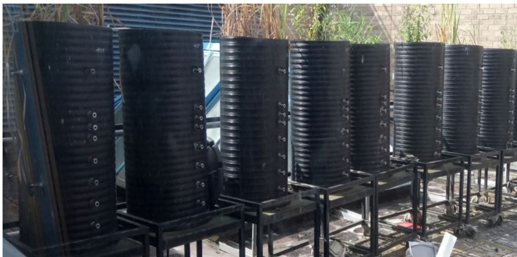
Figure 3-2 Experimental set-up of the pilot-scale VFCWs
