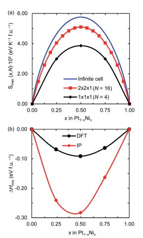
Fig. 1 (a) Maximum configurational entropy ( $S_{max}$ ) for different number of f.u. (N) and (b) mixing enthalpies ( $\Delta H_{\text{mix}}$ ) for the 1  $\times$  1  $\times$  1 supercell both per formula unit of  $Pt_{1-x}Ni_x$  and as a function of the Ni mole fraction (x).  $\Delta H_{\text{mix}}$  was calculated using DFT and IP-based simulations.
