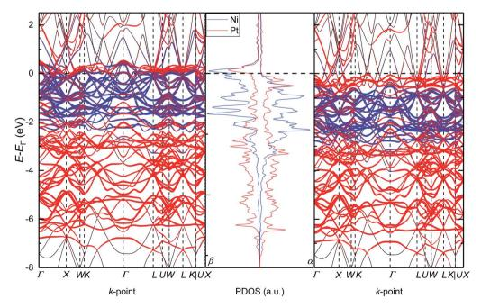
Fig. 5 Electronic density of states and band structure for configuration B of the solid solution with the Pt<sub>0.5</sub>Ni<sub>0.5</sub> composition.  $\alpha$  and  $\beta$  stand for the majority and minority channel of the spins, respectively.
