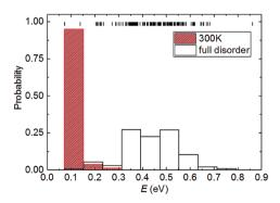
Fig. 2 Partially and fully disordered probability distribution of the energies (E) calculated for the configurations with Ni composition x = 0.50 in the 2  $\times$  2  $\times$  1 supercell. The short vertical lines represent the energy values in the configurational spectrum. The partially disordered probability distribution was calculated using a Boltzmann-modulation at 300 K.
