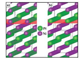
Fig. 3 Schematic representation of configurations (a) B and (b) C for the 2  $\times$  2  $\times$  1 supercell of the solid solution with the  $Pt_{0.5}Ni_{0.5}$ composition. The (110) plane is represented in red.
