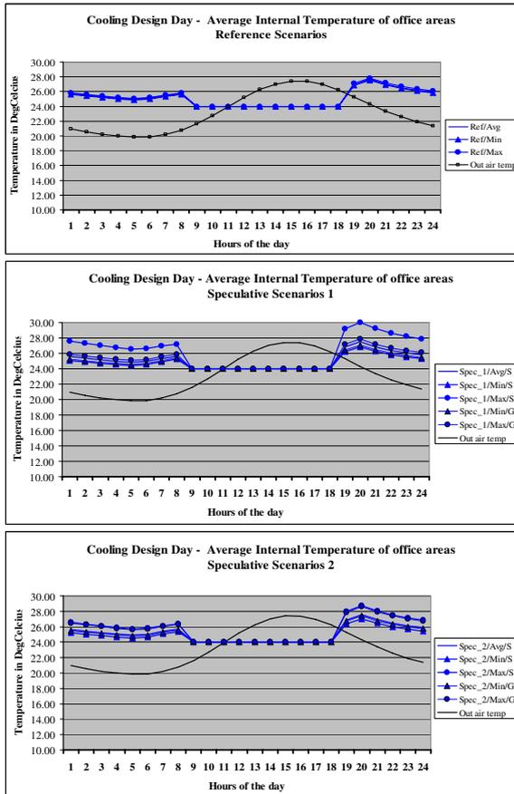
Figure 3 – Hourly average inside temperatures (°C) – Cooling Design Day (CDD)
