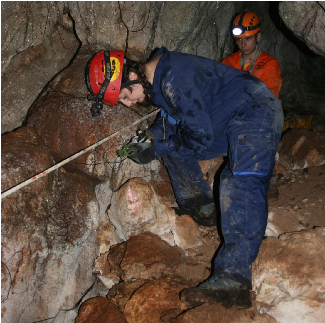
Figure 3 Cave mapping with tape and compass
