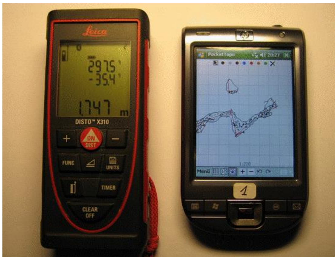
Figure 5 Leica DistoX and PDA with Pocket Topo (image courtesy of B. Heeb)
