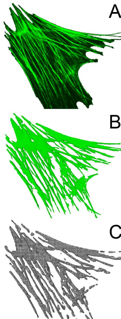
Figure 1: Bovine scleral fibroblast actin stress fiber cytoskeleton 6h after mechanical loading. (A) Confocal laser microscope image; (B) Surface reconstruction in MeshLab; (C) FEM mesh in ABAQUS;
