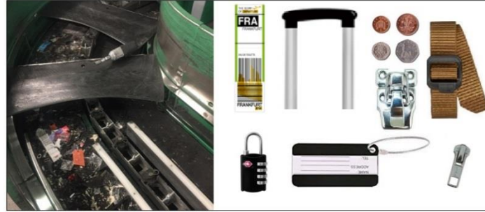
Figure 8: Reclaim carousel survey and items found underneath slats
