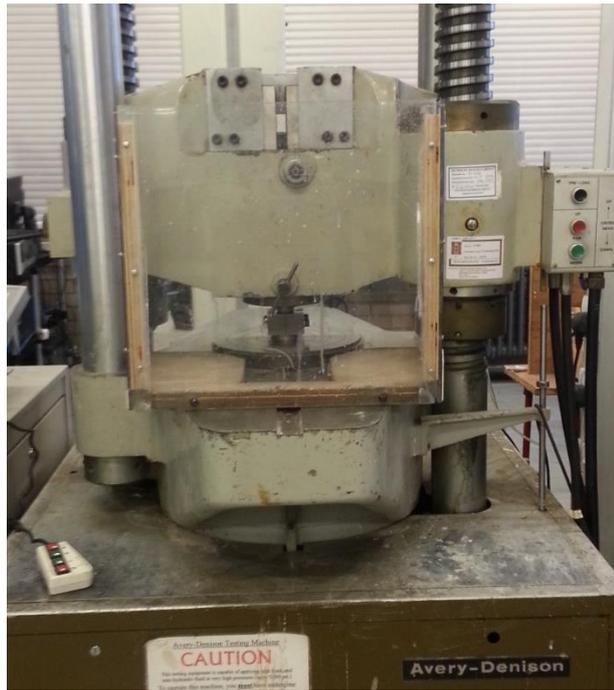
**Figure 5-3 Avery-Denison uniaxial hydraulic operated press. [125]**
