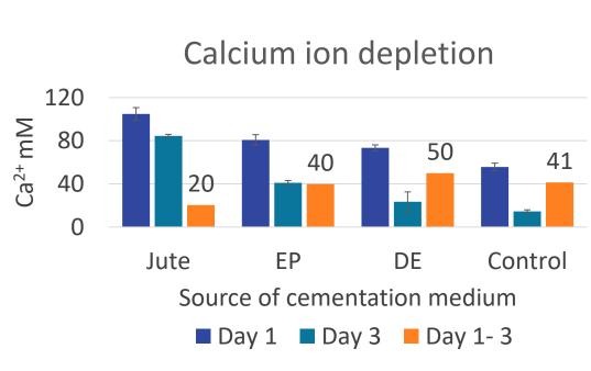
Calcium ion concentration in *S. ureae* inoculated solutions containing cementation medium released from carriers and standard medium as the control, following incubation.
