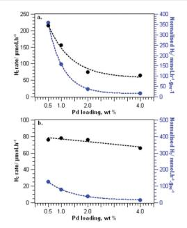
**Fig. 7** Photocatalytic hydrogen generation on  $Pd/TiO_2$  at various Pd loadings. (a) Plot of hydrogen generation rate --- and normalised hydrogen rate ---- against Pd weight loading on the catalyst with a variation of Pd diameter in the range of 2–4 nm. (b) Plot of hydrogen generation rate — and normalised hydrogen rate — against Pd weight loading on the catalyst with a controlled Pd diameter of 3.5 nm.
