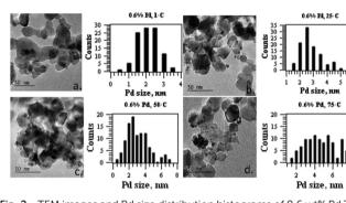
Fig. 2 TEM images and Pd size distribution histograms of 0.6 wt% Pd TiO<sub>2</sub> synthesised at (a) 1 °C, (b) 25 °C, (c) 50 °C and (d) 75 °C.
