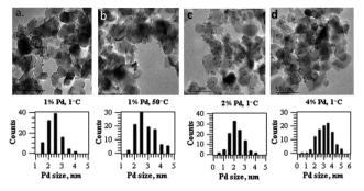
Fig. 4 TEM images and Pd size distribution histograms of (a)  $1\% \text{ Pd/TiO}_2$  synthesised at 1 °C, (b)  $1\% \text{ Pd/TiO}_2$  synthesised at 50 °C, (c)  $2\% \text{ Pd/TiO}_2$  prepared at 1 °C and (d)  $4\% \text{ Pd/TiO}_2$  prepared at 1 °C.
