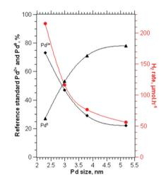
**Fig. 6** Comparison of the catalyst performance in hydrogen production plotted against the size of tailored 0.6% Pd prepared by temperature controlled colloidal synthesis. Percentages of Pd oxidation states derived from normalised XANES spectra were also plotted against the particle size of Pd derived using TEM analysis.
