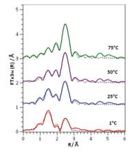
Fig. 1  $k_3$  weighted Fourier transform (magnitude) EXAFS data for the 0.6 wt% Pd/TiO<sub>2</sub> catalysts prepared at 1 °C, 25 °C, 50 °C and 75 °C.
