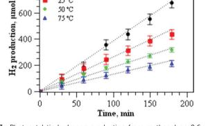
Fig. 3 Photocatalytic hydrogen production from methanol on 0.6 wt% Pd/TiO<sub>2</sub> prepared at different synthesis temperatures.
