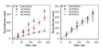
Fig. 5 (a) Photocatalytic hydrogen production from methanol on  $Pd/TiO_2$  prepared at 1 °C at different weight loadings with an average diameter of 2–4 nm; (b) photocatalytic hydrogen production from methanol on  $Pd/TiO_2$  prepared at different weight loadings with an average diameter of 3.5 nm.
