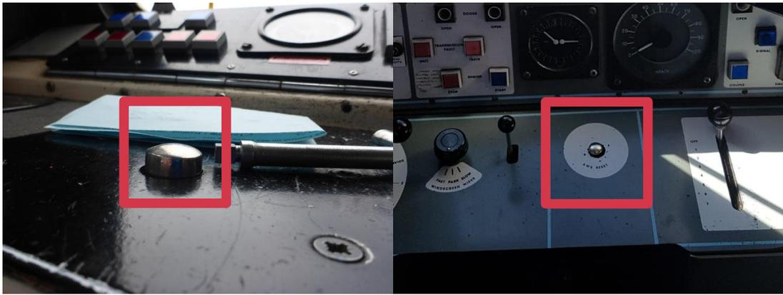
Figure 56: Automatic Warning System (AWS) acknowledgement silver pushbutton below the dashboard
