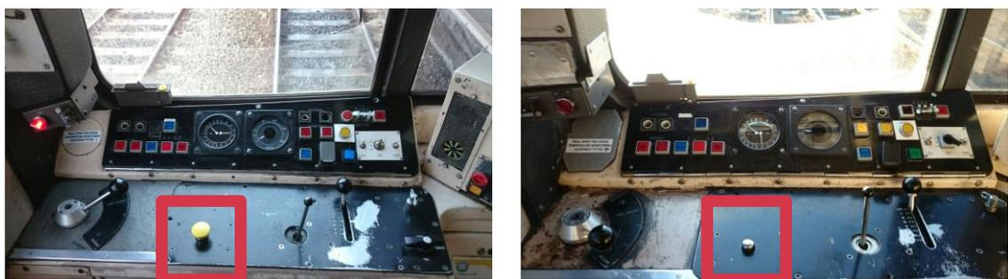
Figure 54: Class 143 cab with different Automatic Warning System (AWS) acknowledgement pushbutton on opposite ends of the same unit
