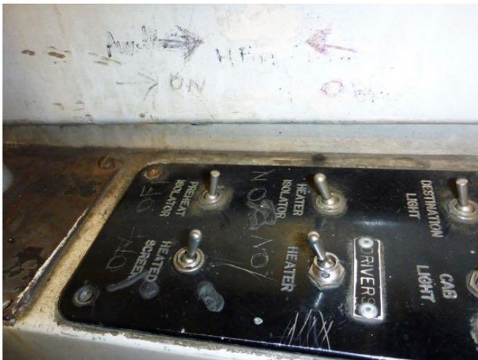
Figure 60: Cab light, destination light and heater setting configuration display
