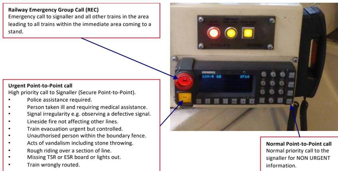
Figure 51: Global System for Mobile Communications – Railway (GSM–R)
