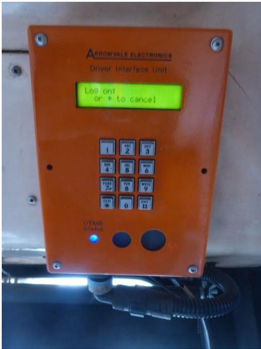
Figure 50: On-Train Monitoring Recorder (OTMR)
