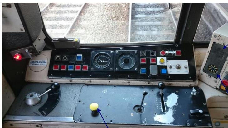
**Automatic Warning System/Train Protection Warning System (AWS/TPWS) Acknowledgement Button**
