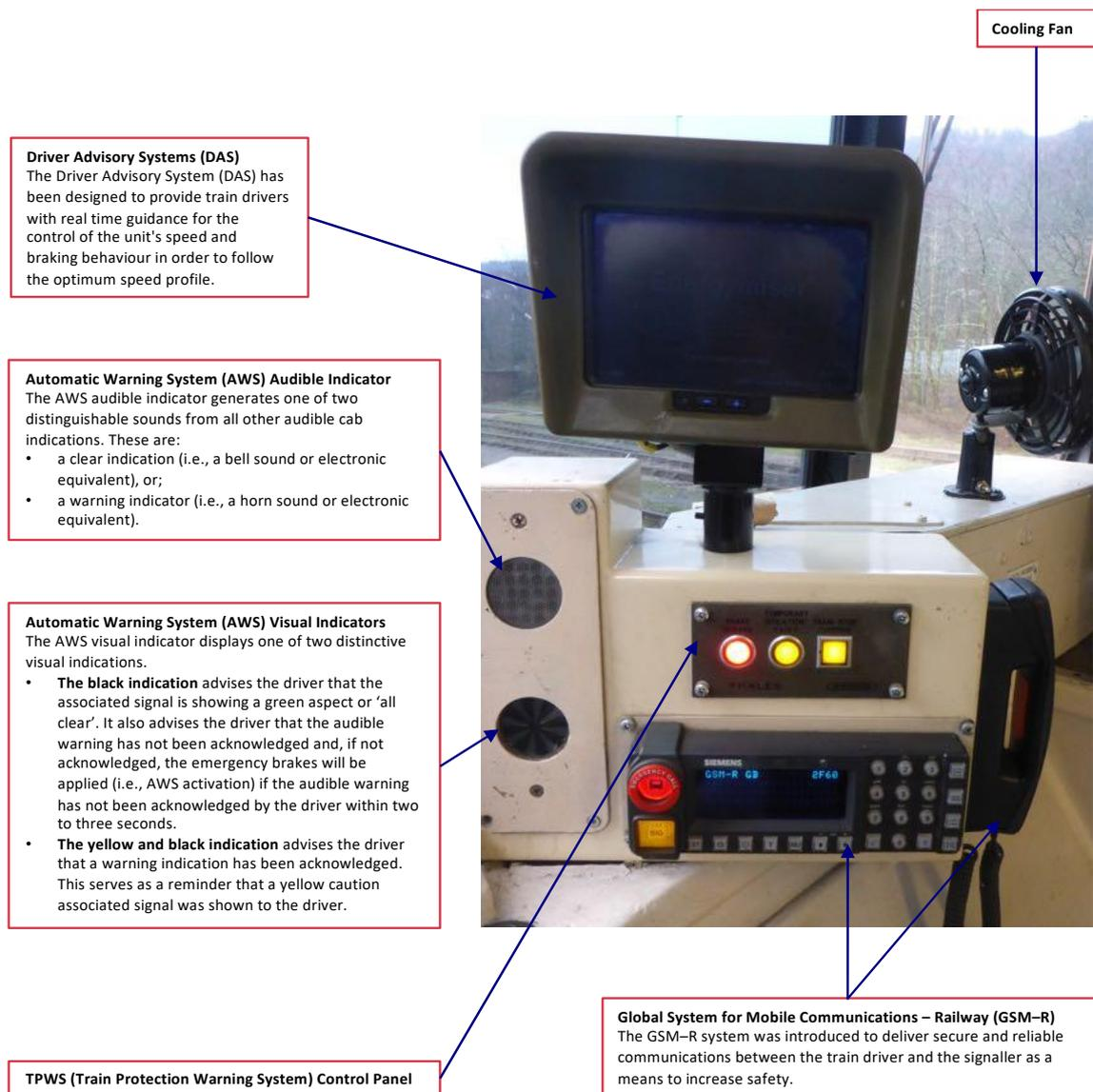
Figure 49: Global System for Mobile Communications – Railway (GSM-R), and Driver Advisory Systems (DAS)
