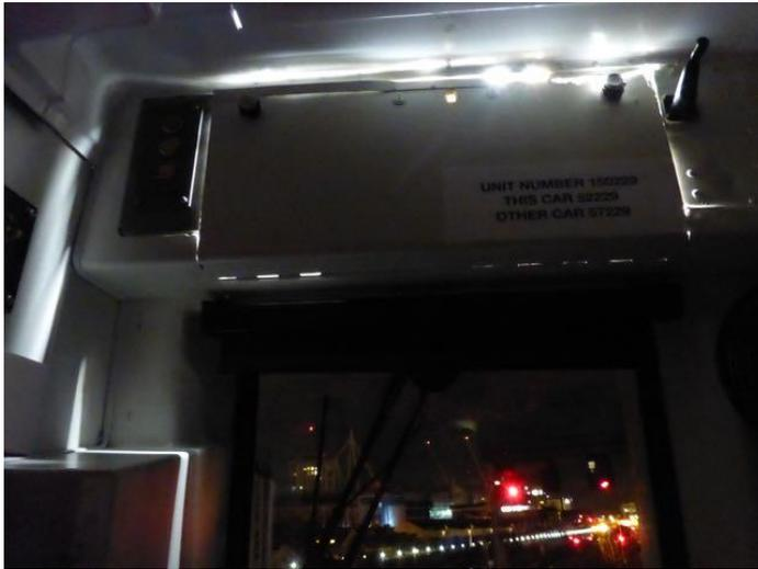
Figure 59: Light contamination from the destination blind
