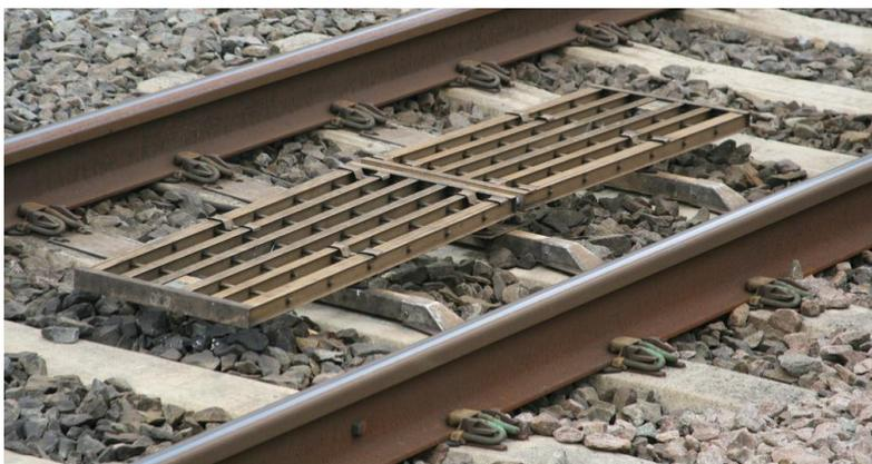
Figure 8: Train Protection Warning System (TPWS)
