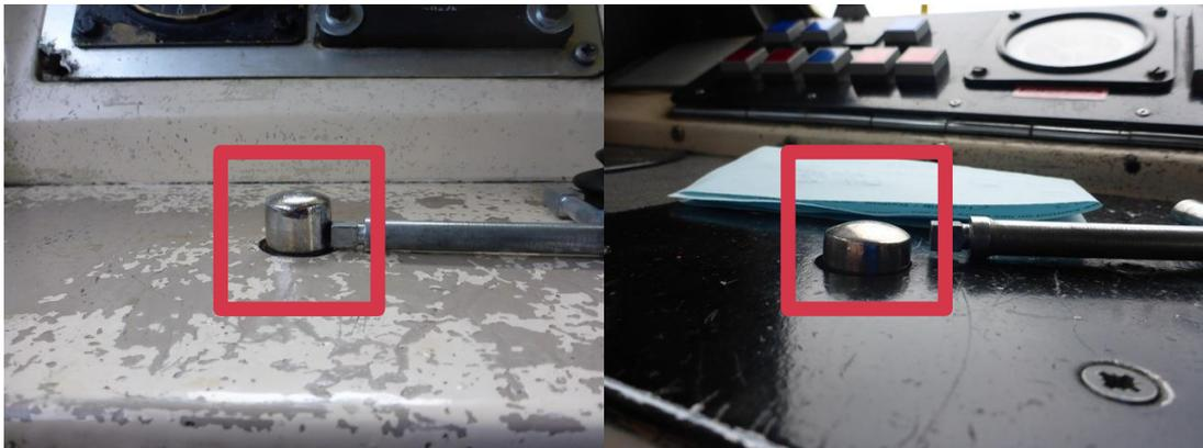
Figure 55: Automatic Warning System (AWS) acknowledgement silver pushbutton position variation
