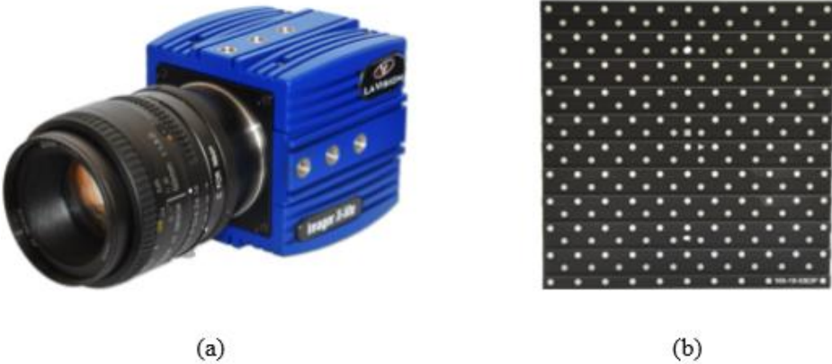
Figure 7.12: (a) LaVision X-lite 8M DIC camera, (b) calibration target plate
