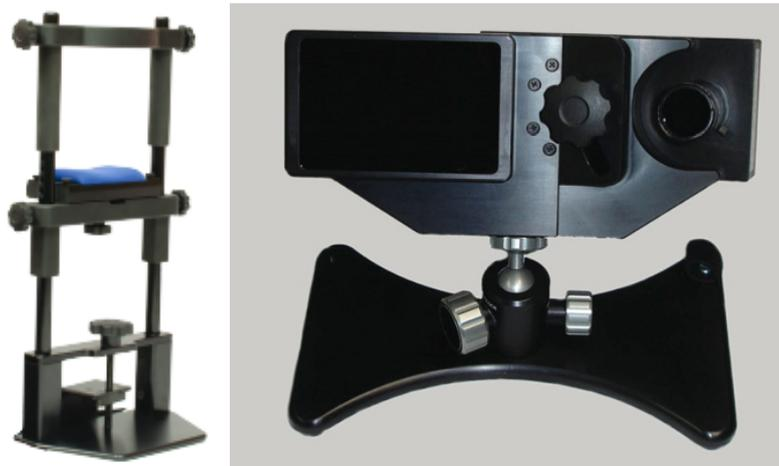
Figure 1.9) is a remote eye tracker with a sampling rate of 1000Hz (monocularly) and 500Hz (binocularly). It has a spatial resolution of 0.1°, and is capable of tracking gaze angles up to 32° horizontally and 25° vertically. It allows head movements within a volume of 25x25x10cm (width x vertical x depth) at a distance between 40cm to 70cm. However, the manufacturers (Research 2014) recommend the use of a chin rest when a spatial resolution is important.
