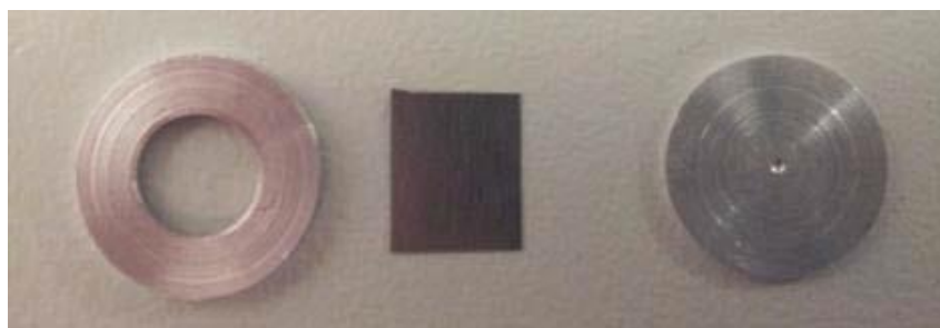
Figure 8-2: Aluminium solid target holder with ^{89}\text{Y} target foil (in the centre)
