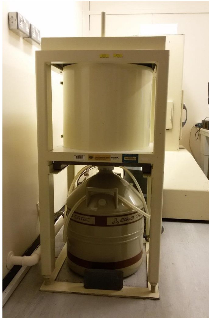
Figure 4-6: HPGe detector at University Hospital of Wales showing the Dewar and shielding
