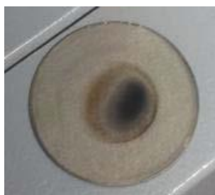
Figure 8-3: Niobium vacuum chamber window for proton energy degradation-the dark area is the beam trace
