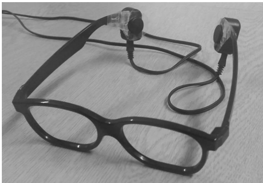
138 FIG 3 Image of lens-less glasses with attached B71 bone transducers.
