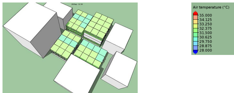
Figure 3. Room air temperature ranges in the formal area for 1 st floors and top floors: a. FRA2EW, b. FRA2NS
