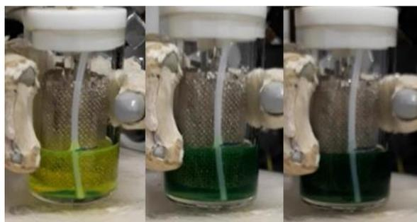
Figure 32 Pictures from the electrolysis experiment demonstrating the colour changes caused by oxidation.
