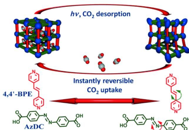
**Figure 1.20** Schematic of the reversible photoinduced CO<sub>2</sub> uptake in Zn-(AzDC)(4,4'-BPE)<sub>0.5</sub>. Taken from reference 95.
