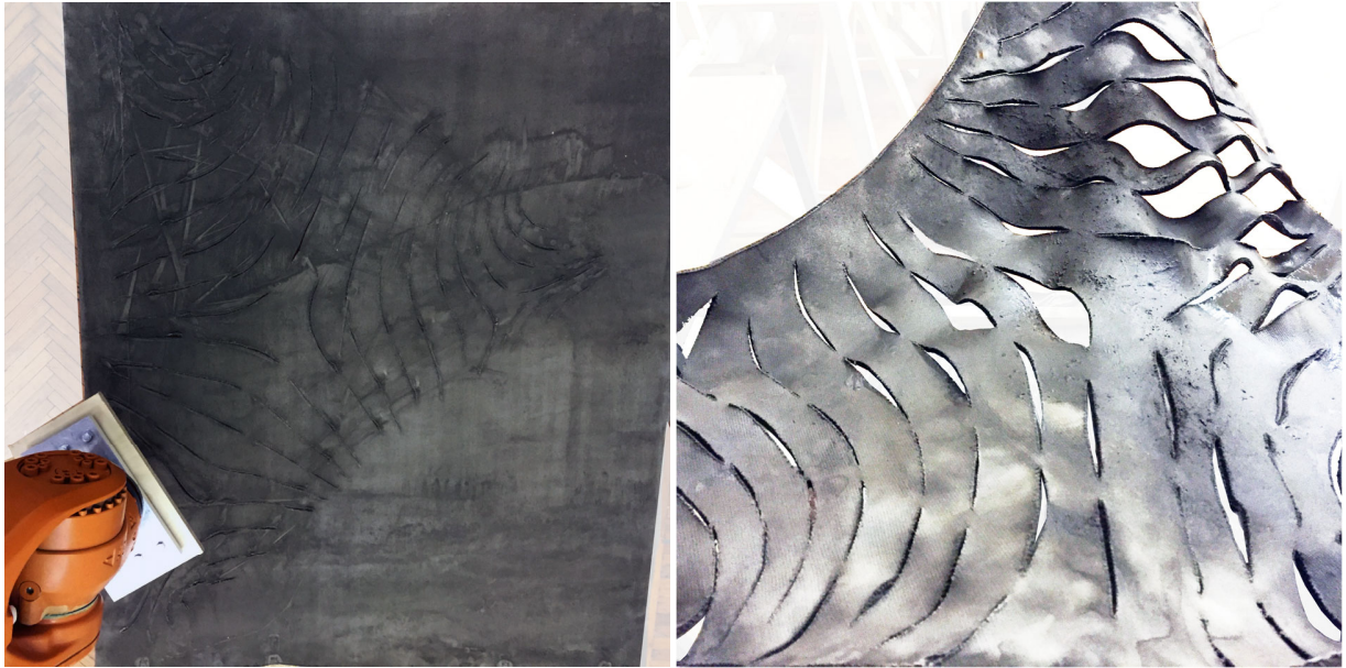
Figure 6-1 . Design process enabled by the robot. Cutting and hydrating the concrete before the forming phase
