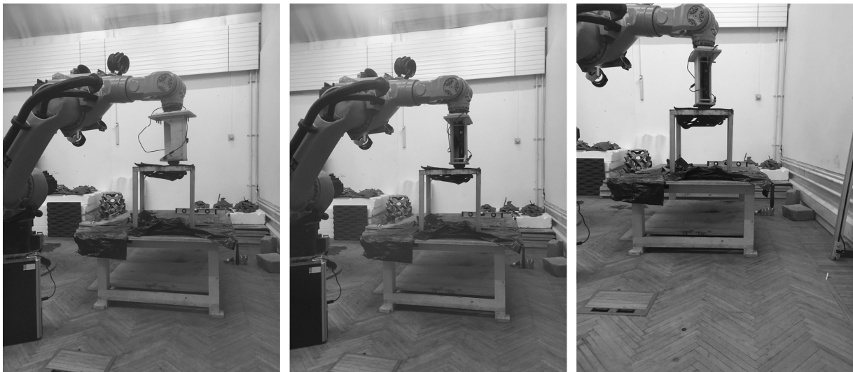
Figure 7-18 Plunging step, including rotation and material massaging at teach plunge.
