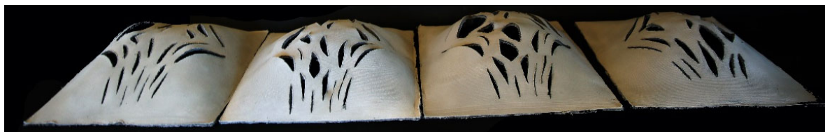
Figure N-0-5 Back view, differences in the 3D pop-up pattern due to the plunging and hydrating sequence.
