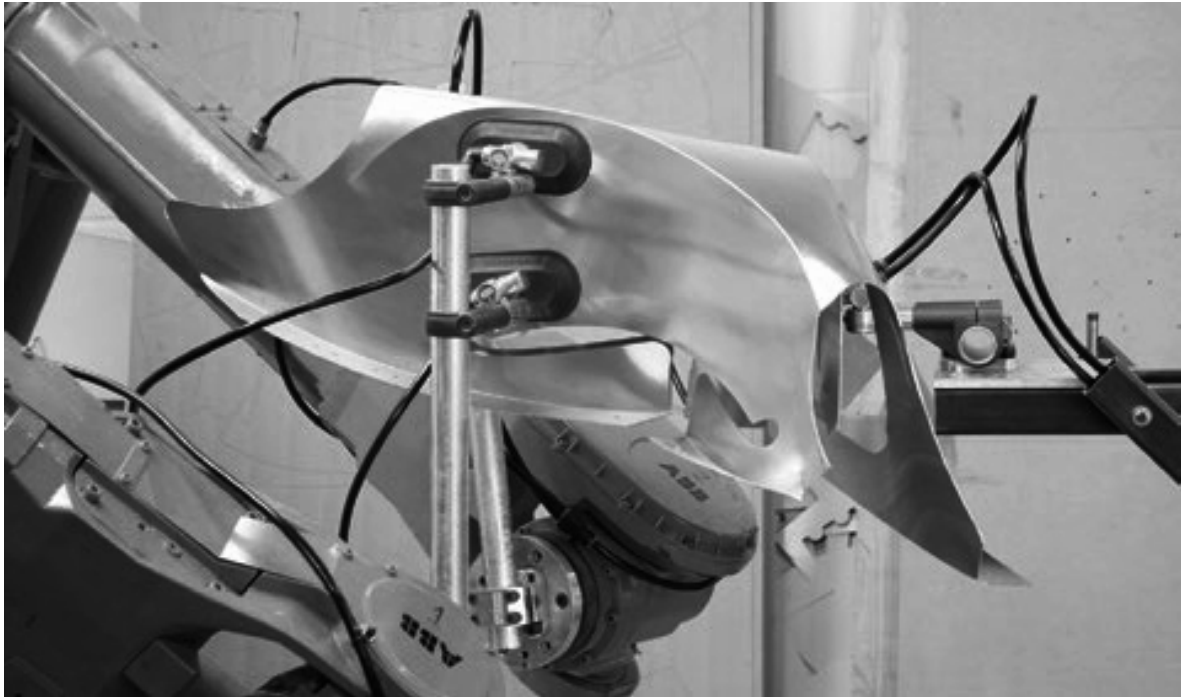
Figure 3-5 Robotic folding process of pieces for 'Arum', Zaha Hadid Architects (Epps 2014).
