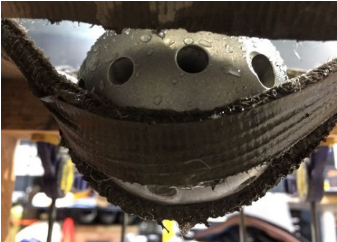
Figure N-0-2 Rotating and hydrating sphere on the opposite side of the end effector
