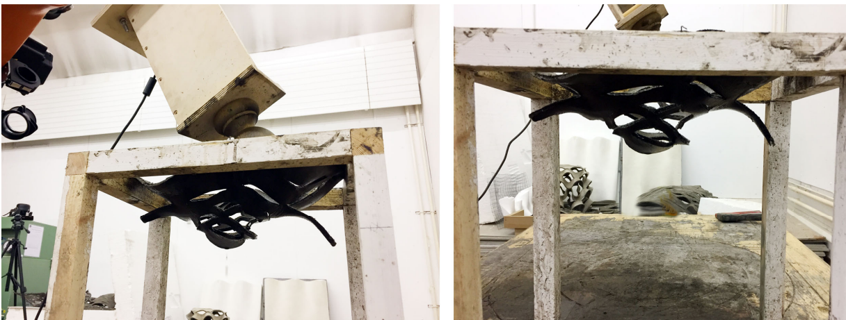
Figure 7-20 Last plunging iteration and concrete fully hydrated, ready for settling.
