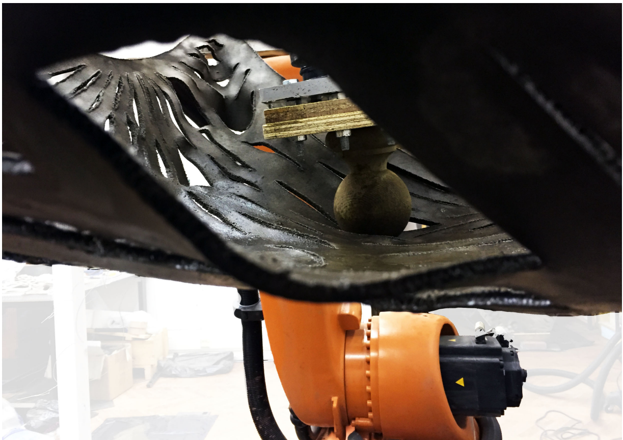
Figure 6-2 Robot plunging and forming the material during the phase-changing stage.
