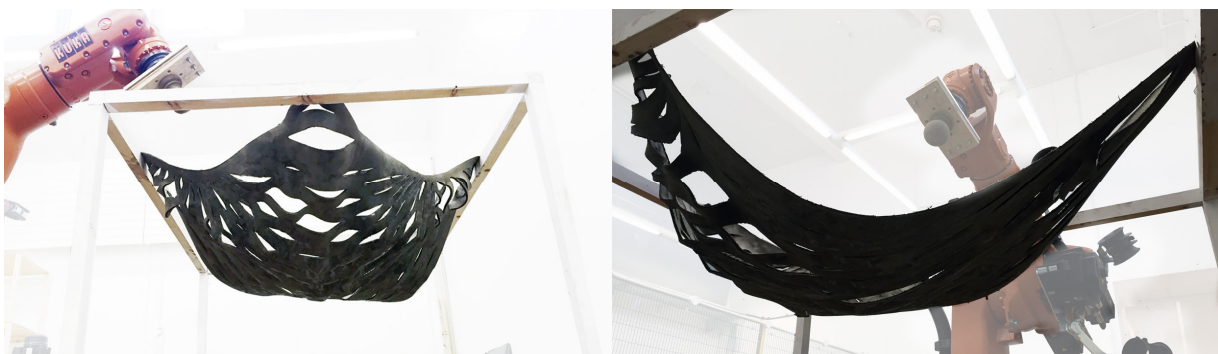
Figure 6-10 Shaping process of concrete based on a predefined pattern of cuts
