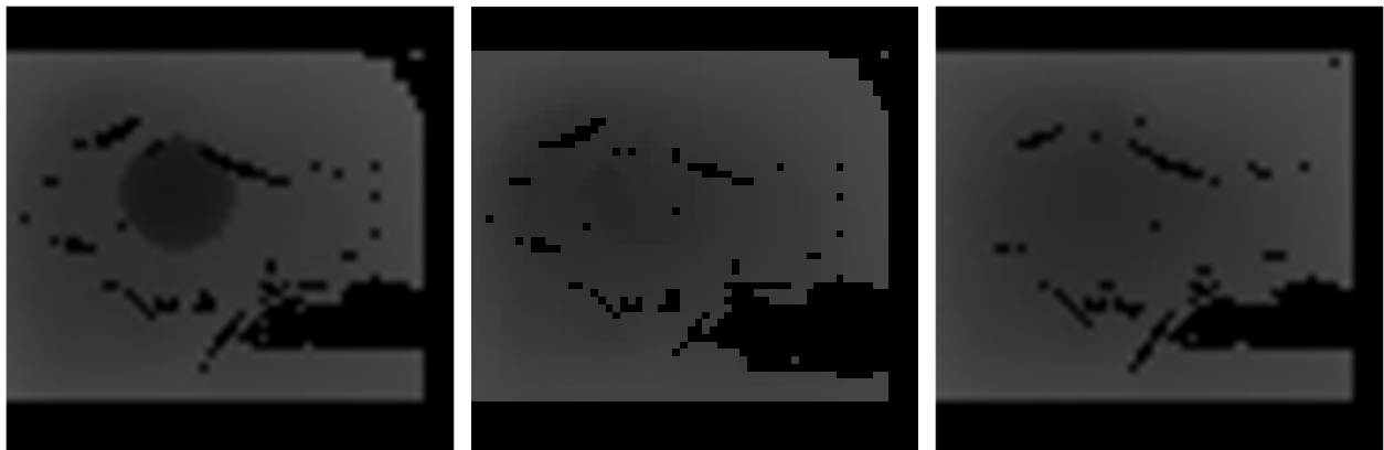
Figure N-0-6 Example of input images from the training data set. Left: Input Image showing the initial condition with the sphere overlap; Middle: actual cloth condition after plunging; Right: Neural Network guess of the resultant shape after plunging.
