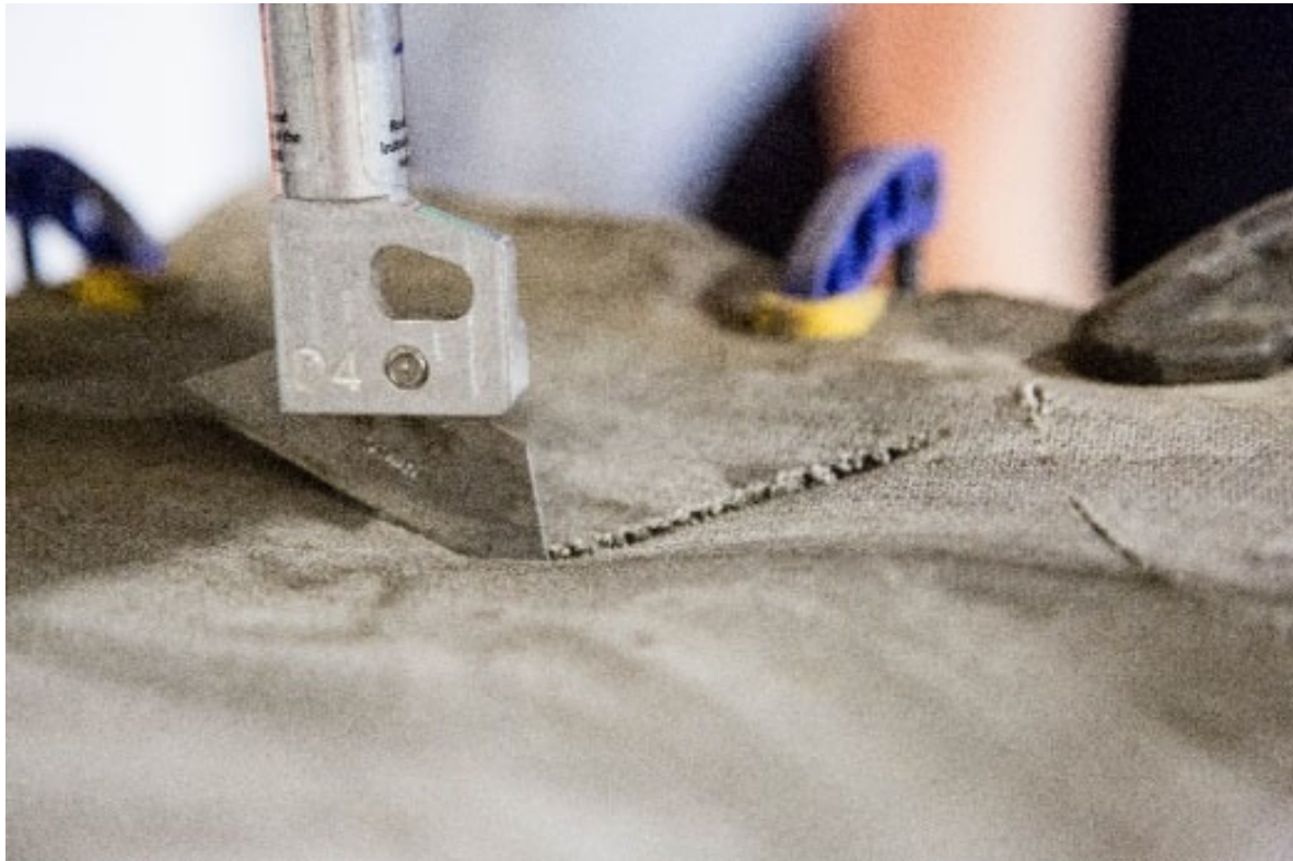
Figure N-0-1 Pivoting knife for cutting the concrete cloth both hanging or on top of a table.
