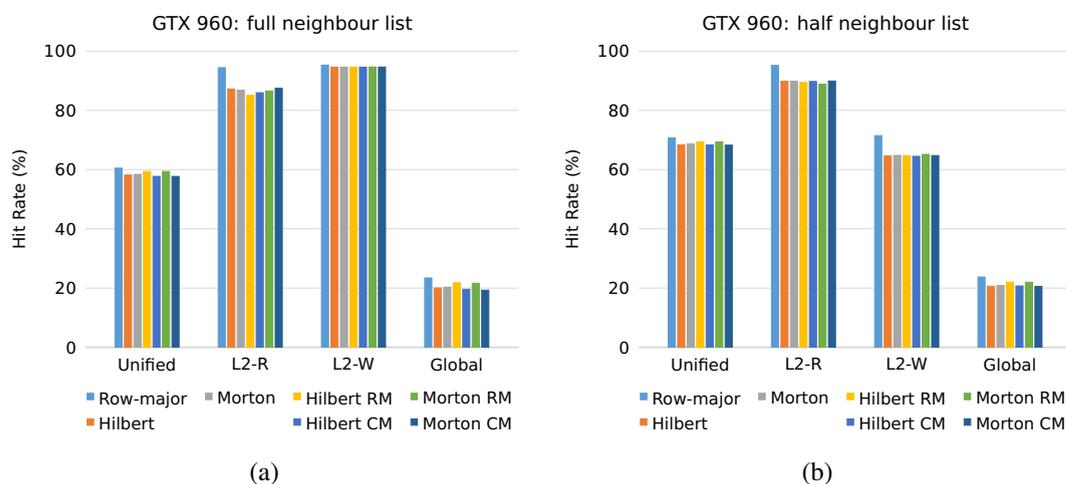
**Figure 6.21: Ruthenium: cache hit rate for the full (a) and half (b) neighbour list algorithms.**
