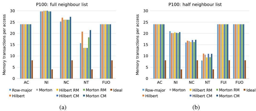
**Figure 6.20: Hawk: number of memory transactions per access for the full (a) and half (b) neighbour list algorithms.**
