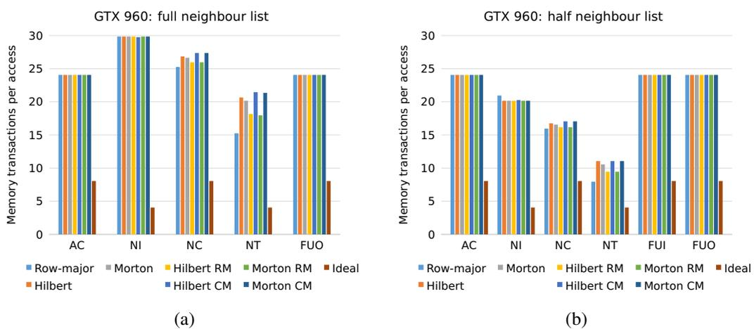
**Figure 6.19: Ruthenium: number of memory transactions per access for the full (a) and half (b) neighbour list algorithms.**
