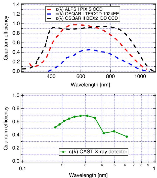
**Fig. 2** Quantum efficiency as a function of the wavelength. Left-hand side panel: the quantum efficiency of the detectors using the method “light shining through a wall”; in the right-hand panel: the quantum efficiency of the Micromegas X-ray detector used in the CAST experiment. The detector bandwidth and their normalised quantum efficiency function are used to compute the upper limits un GWs detectors
