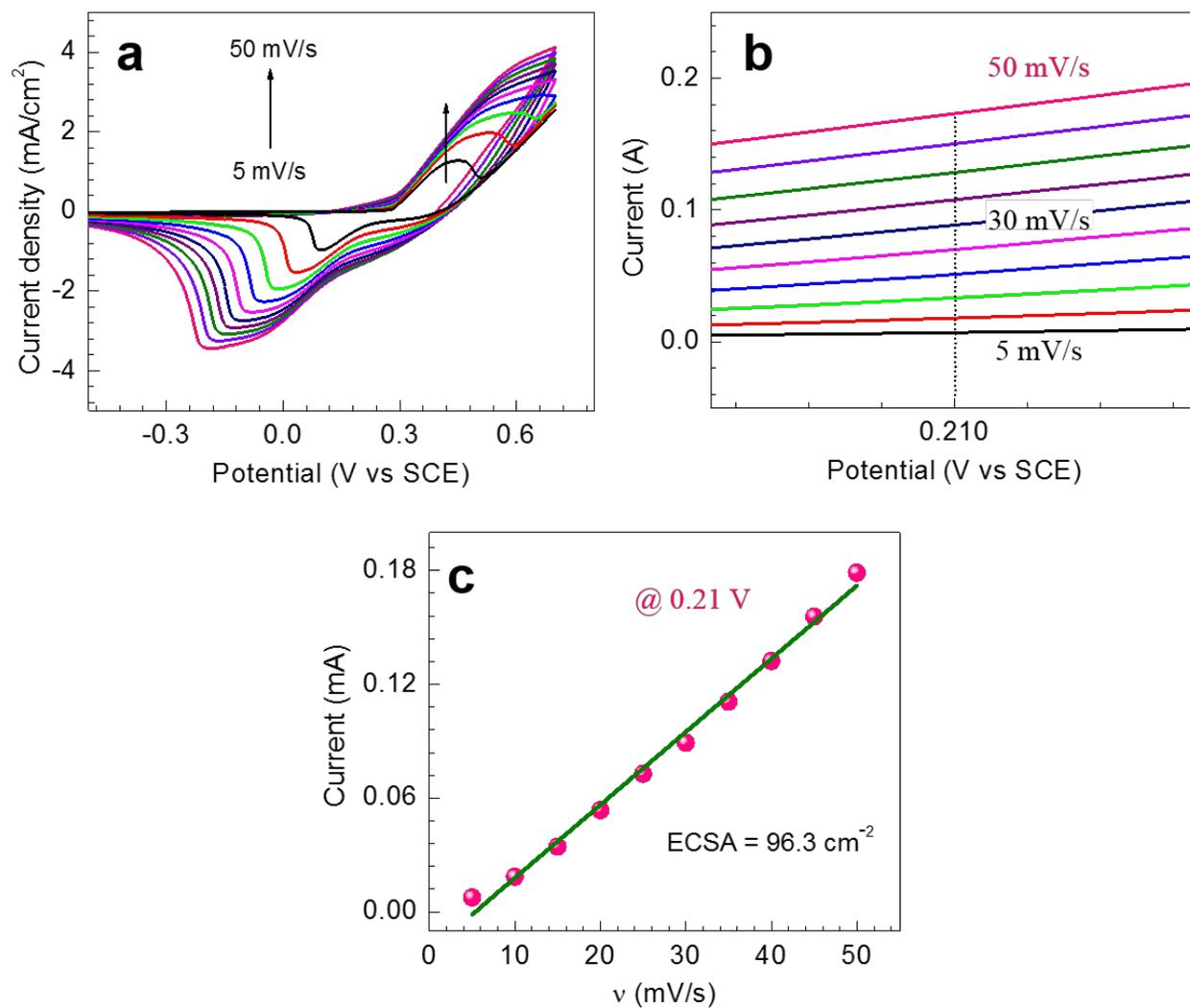
**Fig. 6.** (a) Cyclic Voltammogram (CV) of the NiMoO<sub>4</sub> electrode at various scan rates. (b) Non-faradaic current in the low potential region for various scan rates ( $\nu$ ). (c) Capacitive current ( $I_{DL}$ ) measured at 0.21 V, as a function of scan rate.
