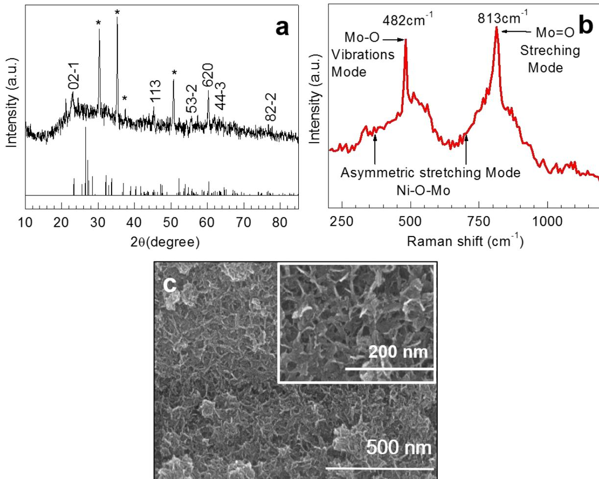
**Fig. 2.** (a) X-ray diffraction pattern of the NiMoO<sub>4</sub> film, along with the standard JCPDS (45-142) data. The star symbol (\*) indicates the signal from the ITO substrate. (b) Raman spectrum of the NiMoO<sub>4</sub> film, showing two main peaks associated with Mo–O vibration and Mo=O stretching modes of the NiMoO<sub>4</sub> structure. (c) SEM image of the NiMoO<sub>4</sub> film, showing a unique nanoflake morphology.
