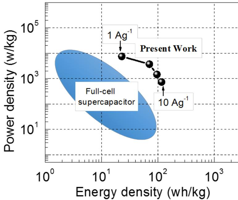
**Fig. 8.** Calculated energy and power densities (Ragone plot) for the NiMoO<sub>4</sub> electrode at various charge/discharge current densities.
