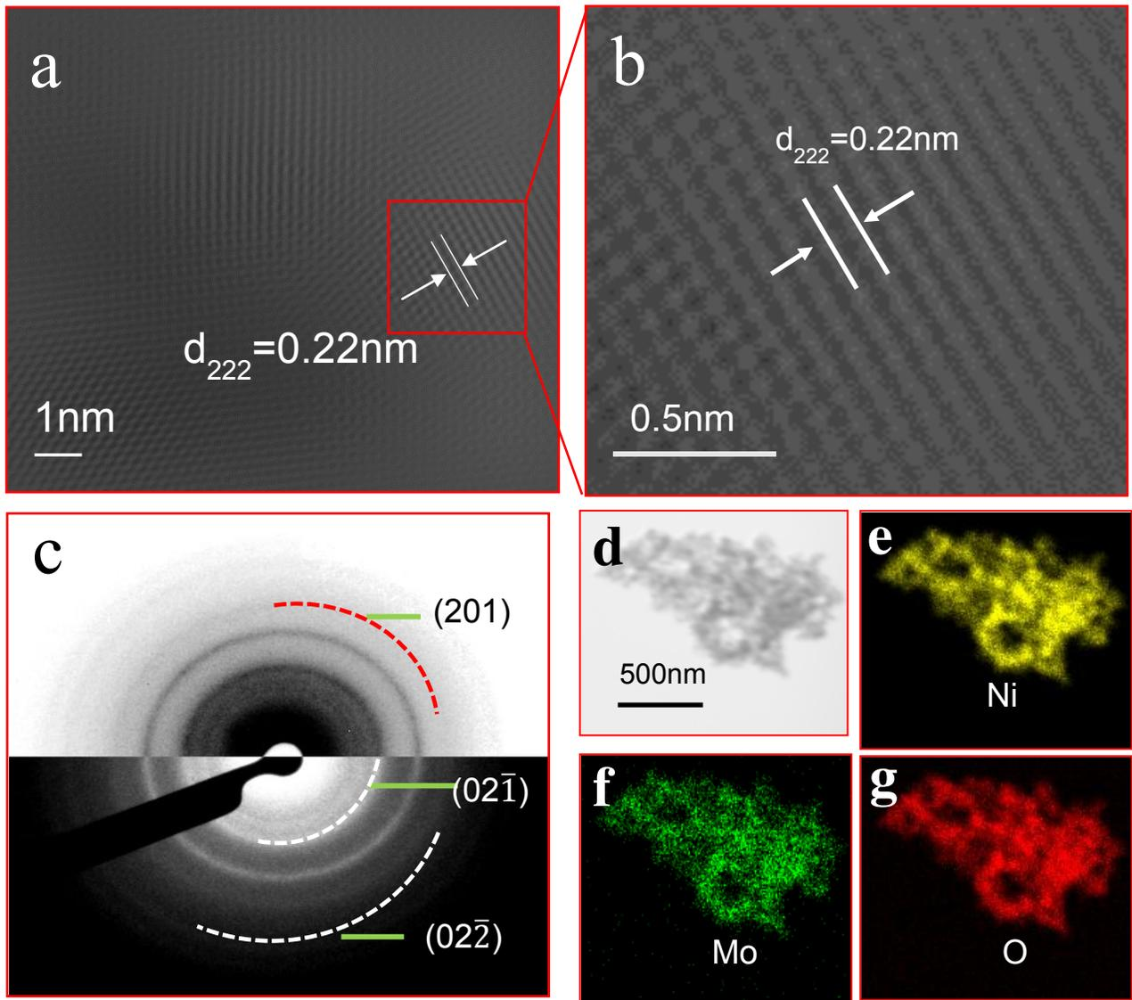
**Fig. 3.** (a) HRTEM image of the nanoflake NiMoO<sub>4</sub>, (b) HRTEM image showing lattice fringes, (c) selective area electron diffraction (SAED) pattern, and (d-g) HAADF-STEM image of nanoflake NiMoO<sub>4</sub> and elemental mapping under the TEM mode, revealing the homogeneous distributions of Ni, Mo, and O in the nanoflake NiMoO<sub>4</sub>.
