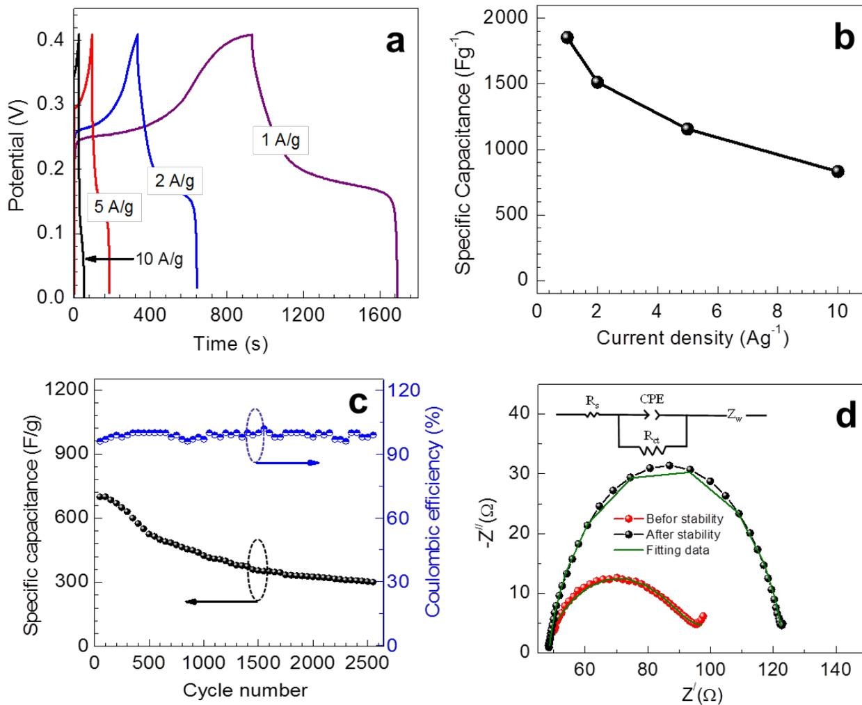
**Fig.7.** (a) Galvanostatic charge-discharge (GCD) curves of the NiMoO<sub>4</sub> electrode at various current densities. (b) Specific capacitance, obtained from the GCD curves at various current densities. (c) Cycling stability test at a high current density of 10 Ag<sup>-1</sup>. (d) Nyquist plot before and after the cycling test.
