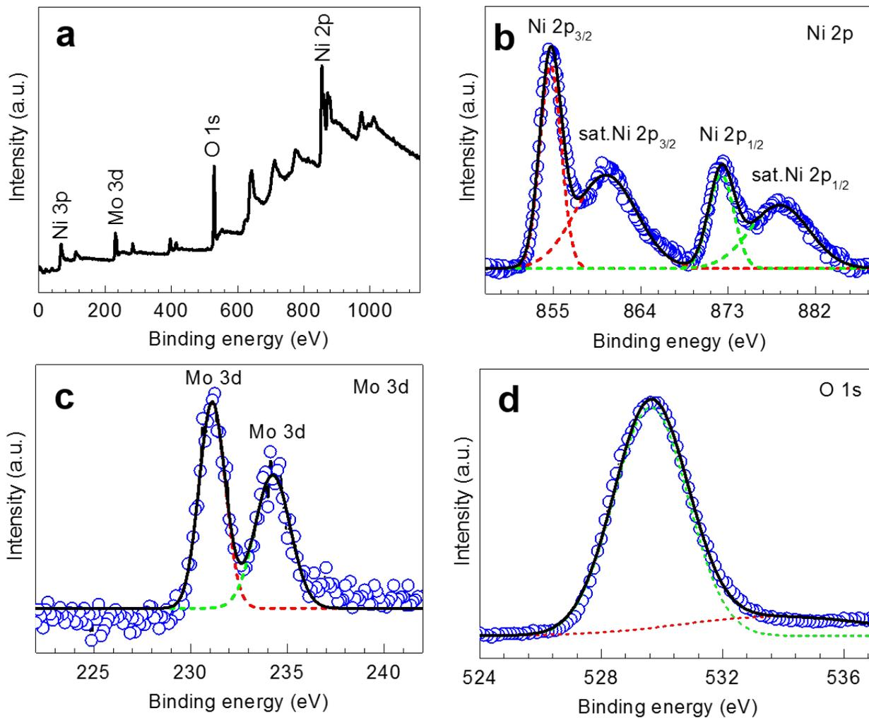
**Fig. 4.** XPS spectra of NiMoO<sub>4</sub>: (a) Survey scan revealing the existence of Ni, Mo, and O as constituent elements. A high-resolution scan of the (b) Ni 2p peaks, (c) Mo 3d peaks, and (d) O 1s peaks. The solid circles and lines represent the experimental data and fitting curves, respectively.
