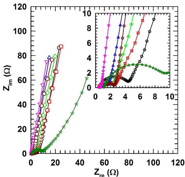
**Fig. 8.** Nyquist plots of the Ni(OH)<sub>2</sub>-POV thin film electrodes. (circle) LNHV-3, (square) LNHV-2.5, (diamond) LNHV-2, (triangle-up) LNHV-1.5, (triangle-down) LNHV-1, (hex) LNHV-0.5, and (star) LNHV-0. The inset shows an enlarged view of the EIS spectra in the high frequency region.
