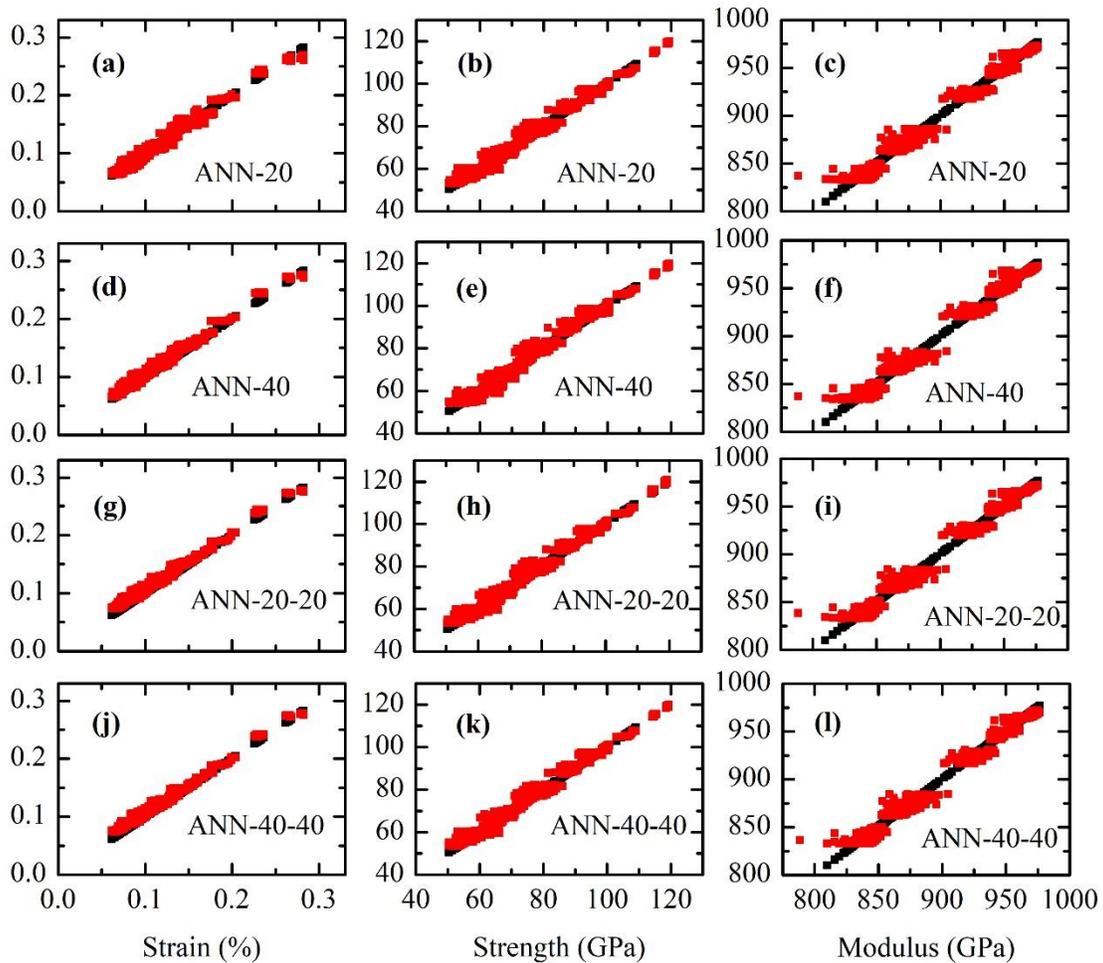
**Figure 9.** Training results of (a)-(c) 1 layer neural network with 20 neurons, (d)-(f) 1 layer neural network with 40 neurons, (g)-(i) 2 layers neural network with 20 neurons each and (j)-(l) 2 layers neural network with 40 neurons each.
