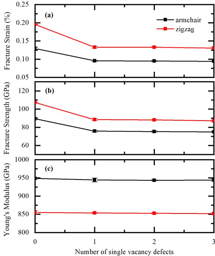
**Figure 6.** Effects of single atom vacancy defect on (a) fracture strain, (b) fracture strength and (c)
