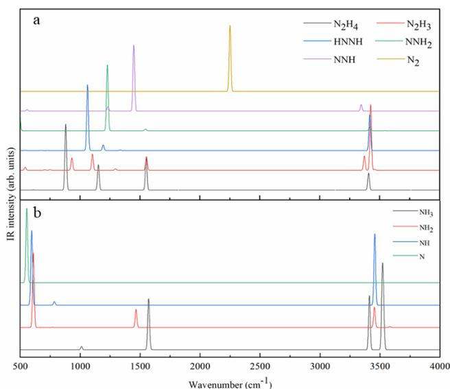
**Figure 16.** a) Infrared spectra for adsorbate N<sub>2</sub>H<sub>4</sub>, N<sub>2</sub>H<sub>3</sub>, HNNH, NNH<sub>2</sub>, NNH and N<sub>2</sub>); b) Infrared spectra for adsorbate NH<sub>3</sub>, NH<sub>2</sub>, NH and N
