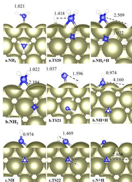
**Figure 12.** Top and side views of the initial, transition and final states for NH<sub>3</sub> dehydrogenation, (a) NH<sub>3</sub> decomposition, (b) NH<sub>2</sub> decomposition (c) NH decomposition. All inset distances are in Å. Blue spheres represent N atoms, white is hydrogen, and Ir is the large green sphere.
