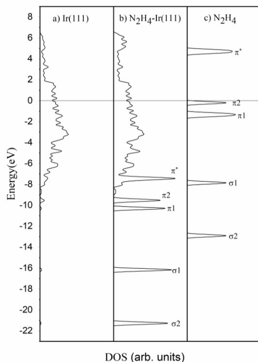
**Figure 7.** The total density of states of a) bare Ir(111), b)  $\text{N}_2\text{H}_4/\text{Ir}(111)$  and c) isolated gauche  $\text{N}_2\text{H}_4$ . The horizontal line across diagrams represents the common Fermi energy.
