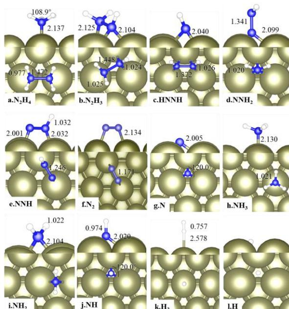
**Figure 5.** Side and Top view of adsorbed N<sub>2</sub>H<sub>x</sub> (x = 0-4), NH<sub>x</sub> (x = 0-3) and H species on the Ir(111) surface (side view and top view). All distances inset are in Å. Blue spheres represent N atoms, white is hydrogen, and Ir is the large green sphere.
