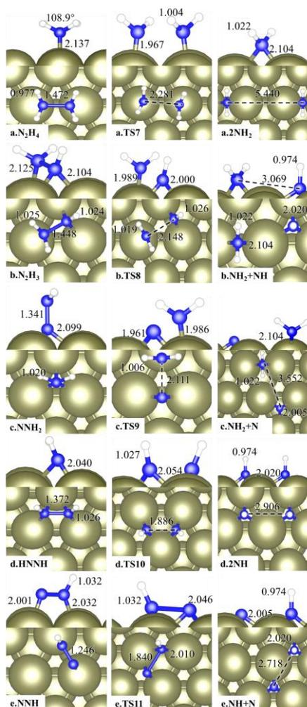
**Figure 9.** Top and side views of the initial, transition and final states for the dissociation pathway of (a)  $N_2H_4$ , (b)  $N_2H_3$ , (c)  $NNH_2$ , (d)  $HNNH$  and (e)  $NNH$ . All inset distances are in Å. Blue spheres represent N atoms, white is hydrogen, and Ir is the large green sphere.
