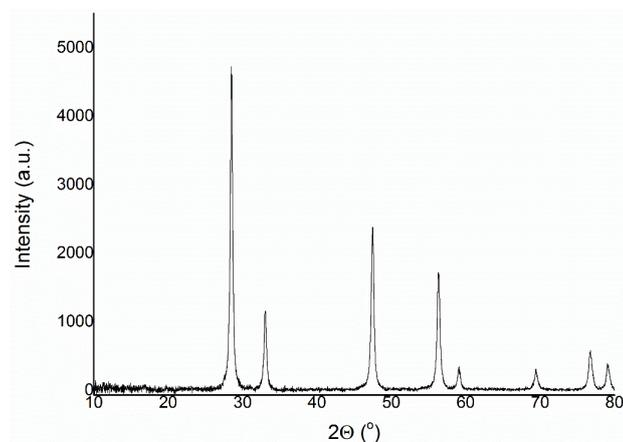
**Figure 2.** X-Ray diffraction pattern for Ir/CeO<sub>2</sub>
