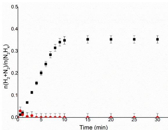
**Figure 4.**  $n(\text{H}_2+\text{N}_2)/n(\text{N}_2\text{H}_4)$  versus time for hydrous hydrazine decomposition over  $\text{Ir}/\text{CeO}_2$  using 0.3mL of 3.3M hydrazine monohydrate in 8mL 0.5M of NaOH solution, at  $50^\circ\text{C}$  and 76.2 mg of catalyst, for a substrate/metal ratio of 250, with a stirring rate of 1050 rpm. Black squared measurements correspond to reduced samples, while red circles indicate the non-reduced sample.
