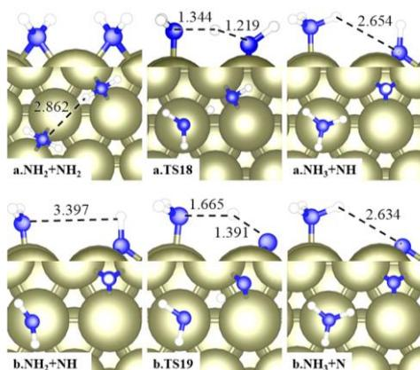
**Figure 11.** The top and side view of the initial, transition and final states for the interaction of NH<sub>2</sub> molecules. (a) NH<sub>2</sub> and (b) NH. All inset distances are in Å. Blue spheres represent N atoms, white is hydrogen, and Ir is the large green sphere.
