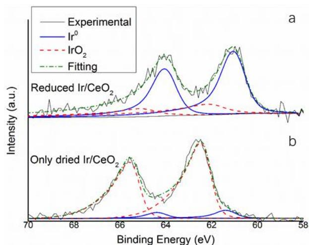
**Figure 3.** XPS spectrum of Ir 4f region for Ir/CeO<sub>2</sub> with deconvolution for metallic Ir and
