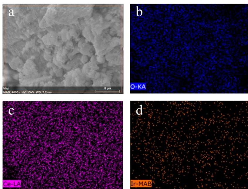
**Figure 1.** a) SEM image of Ir/CeO<sub>2</sub>, b-d) the EDS mapping of its surface for the main element present in the catalyst.
