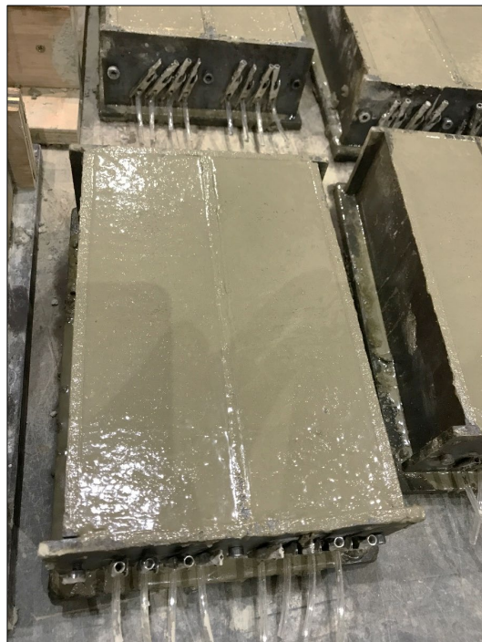
Figure 3.3. Specimen preparation for Groups A and B with twin moulds after casting
