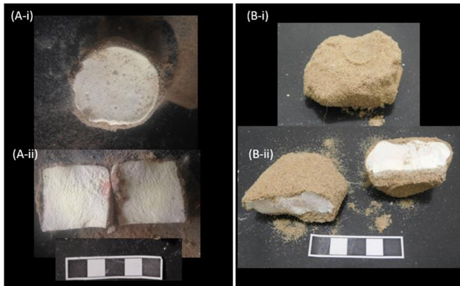
Figure 6.14. Example of samples in which no fractures formed. (i) top surface of dried corn-starch patties (ii) broken vertically in half to reveal no internal fracture patterns. For (A) sample 45 and (B) sample 48. Scale bar 5 cm.
