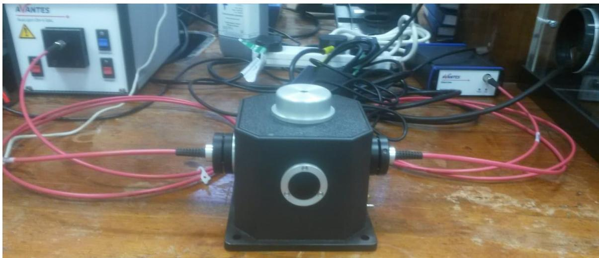
Figure 2.14. (Up-left) AvaLight-DH-S deuterium halogen source, (up-right) AvaSpec-ULS2048XL EVO spectrometer and (bottom) CUV-UV/VIS-TC temperature-controlled cuvette holder.
