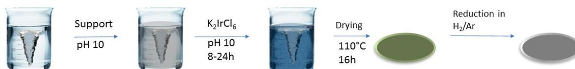
Figure 2.3. Schematic representation of the deposition-precipitation method with NaOH for Ir catalysts used in this thesis, particular importance is covered by the reaction under stirring at controlled pH.
