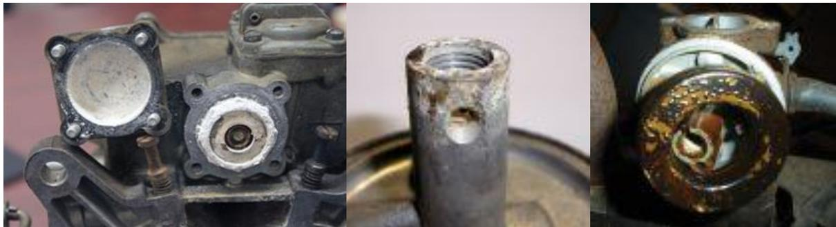
**Figure 1.10:** Effects of ethanol in engines.
