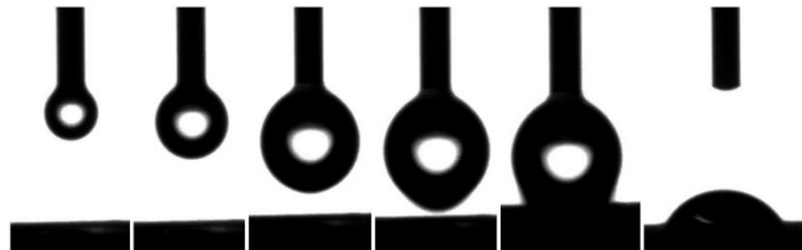
Fig. 3. The process of placing a liquid droplet on a sample surface
