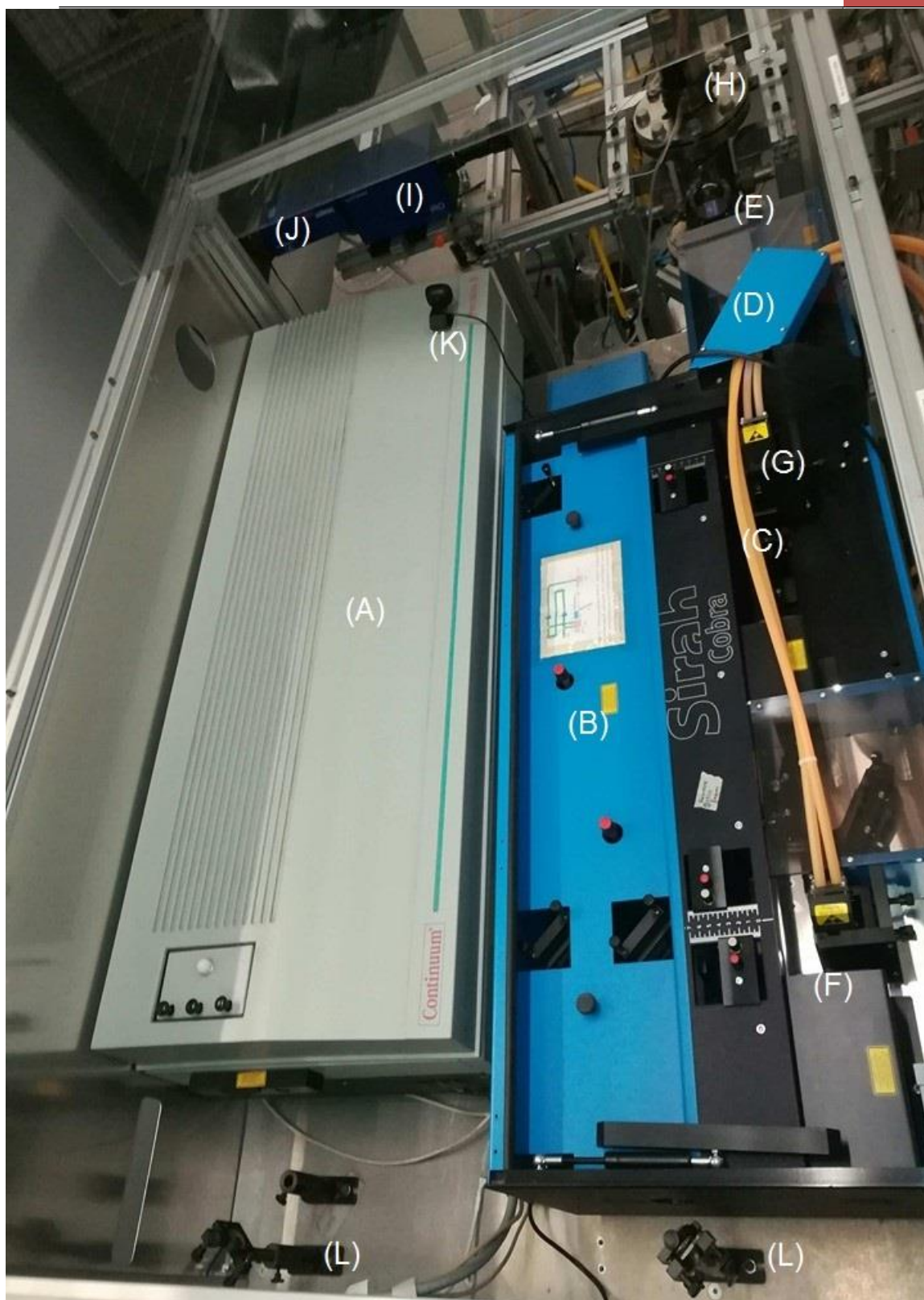
Figure 3.15 PLIF top view, (A: Nd:YAG laser), (B: Dye laser), (C: Rhodamine 6G dye powder and ethanol), (D: Temperature monitor), (E: Sheet forming optics), (F: Grating), (G: Frequency-doubling crystal), (H: burner quartz), (I: IRO intensifier) –(J: CCD camera), (K: Webcam), (L: 45° mirror)
