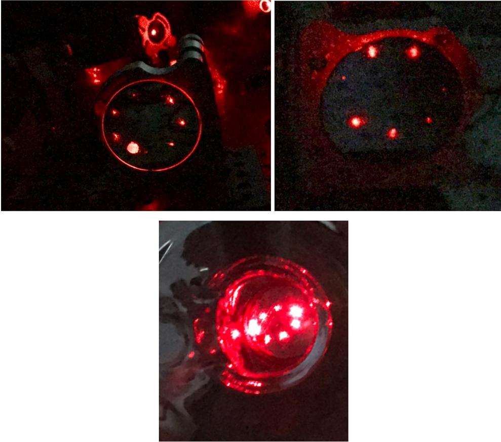
*Figure 105 Spot patterns traced by the red diode alignment beam on the surfaces of the aluminium alignment mirror (top left), the opposing cavity mirror (top right) in optic mounts from initial optical cavity testing, and on the surface of the secondary cavity mirror mounted in the sample chamber (bottom).*
