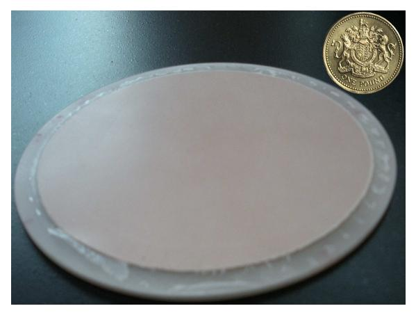
Fig. 5.8 Photograph of the anti-reflection coated BLAST-Pol HWP.
