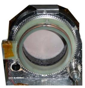
(b) This side of the rotator faces the window of the optics box, about 19.1 cm away on the optical path. Visible in the photograph are the potentiometer, the gear train with the pinion assembly, and the back side of the blackened baffle, which is secured by one screw at the top of the stator, and two more on the 4 K stage. On the left side is visible the encoder readout assembly with the leaf springs.
