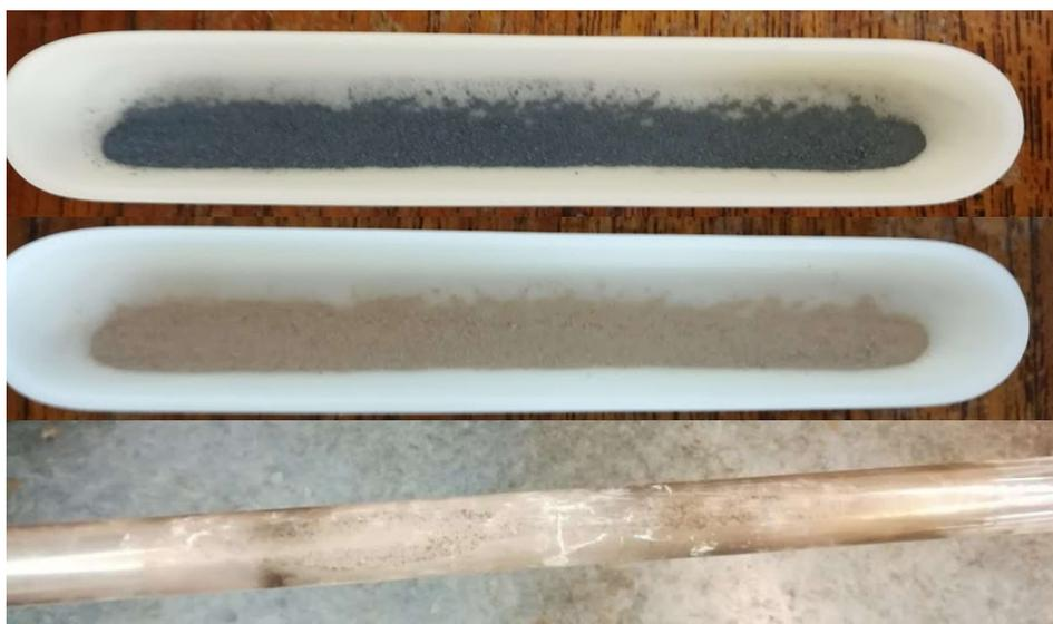
**Figure 32** – Photos of a Pd/TiO<sub>2</sub> catalyst before any heat treatment (top) and after the calcination step (middle) and of the furnace tube used for the reduction step (bottom).
