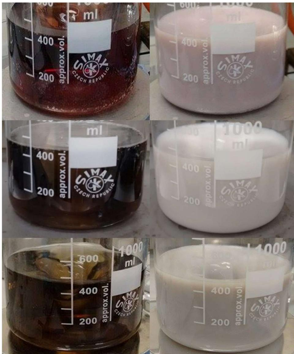
**Figure 14** – Photos of the colloids formed after addition of NaBH<sub>4</sub> (left) and of the support addition stage with TiO<sub>2</sub> (right) for the synthesis of Au (top), Pd (middle), AuPd (1:1 molar) (bottom) catalysts.
