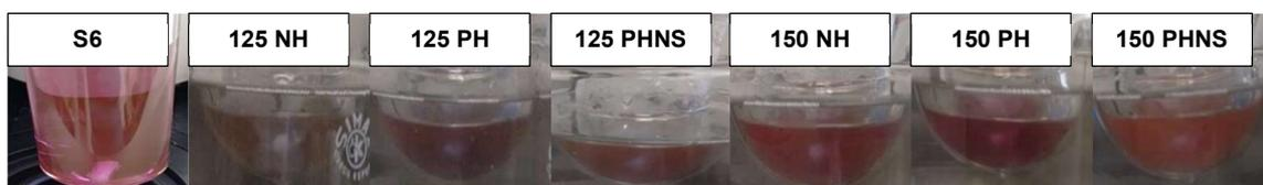
**Figure 48** – Au nanoparticles produced by conventional heating at 125 °C (left) and 150 °C (right) with UV-Vis analysis and photos (bottom) for microwave standard conditions (S6) and for the colloids at 15 min at 125 °C and 150 °C with normal heating (NH), preheating (PH) and preheating no stabilizer (PHNS).
