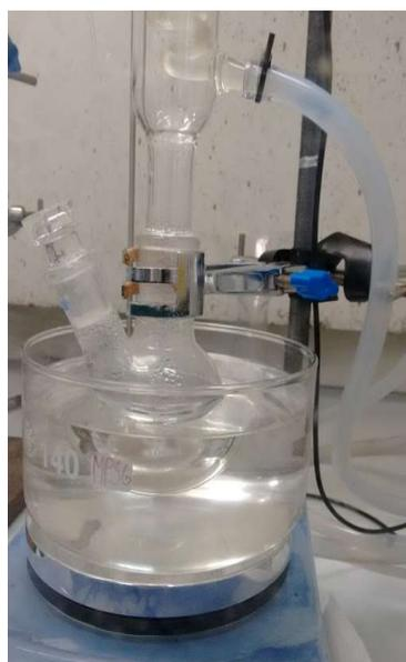
**Figure 36** – Formic acid decomposition reaction experimental set-up.
