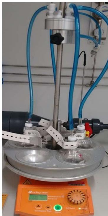
**Figure 35** – Cinnamaldehyde hydrogenation reaction experimental set-up.
