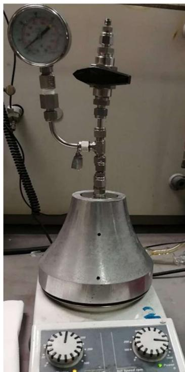
**Figure 34** – Furfural hydrogenation reaction experimental set-up.
