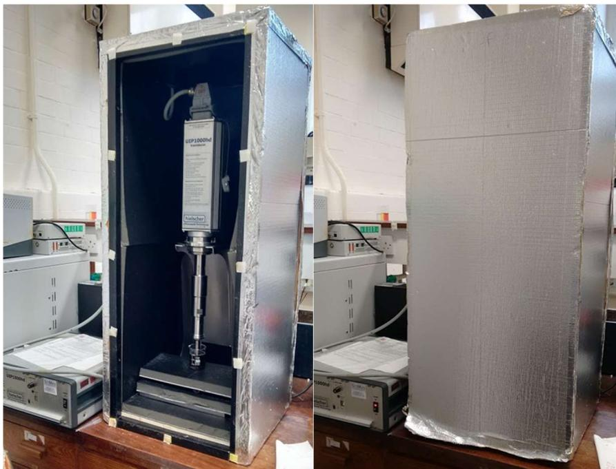
**Figure 29** – Ultrasound synthesis experimental set-up used under batch regime.
