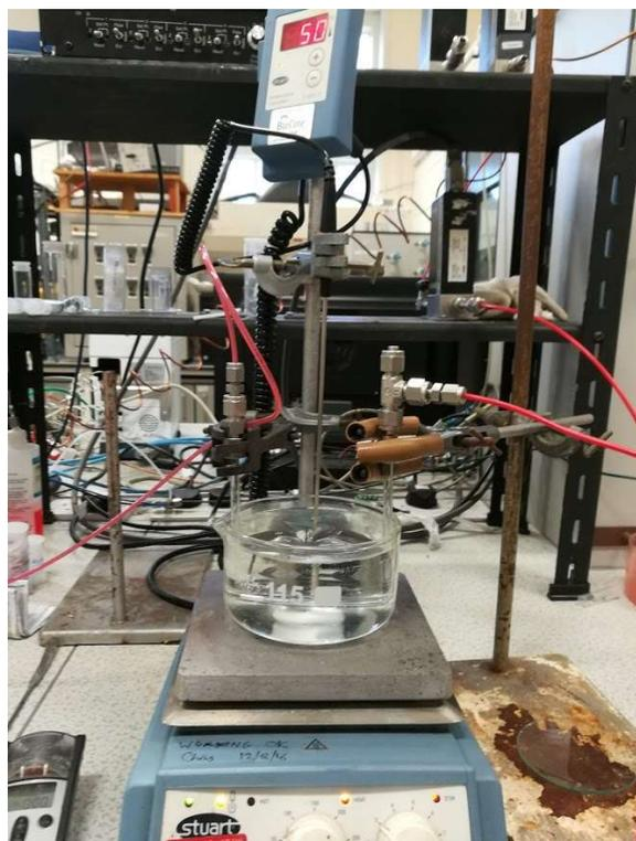
**Figure 33** – Carbon monoxide oxidation reaction experimental set-up.
