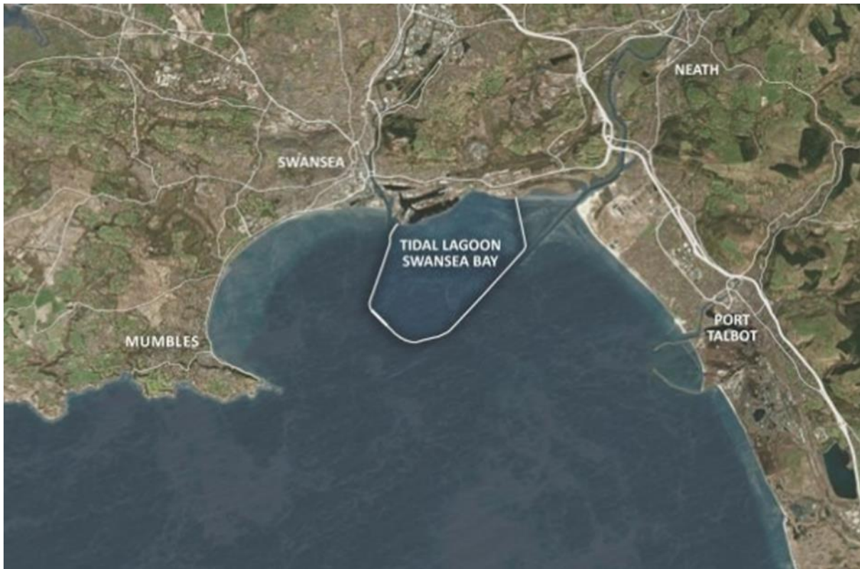
Figure 6.5 – Proposed location of the tidal lagoon within Swansea bay. Note – the gatehouse housing the turbines appears as a slightly thicker white line along the lagoon wall.
