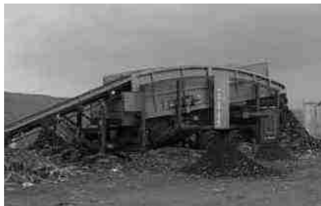
Figure 5. Ballistic separator used in the TönsLM project (Maul et al, 2014)
