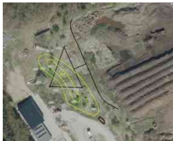
Figure 16. Interpretation of methane diffusion, respectively. >50 vol % and >5 vol %
