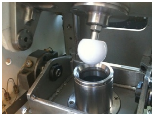
Figure 56 ProSim Hip Joint Friction Simulator
