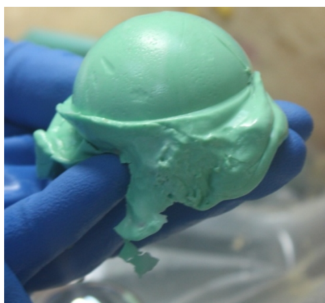
Figure 30 Example dental putty mould of an impacted PEEK cup
