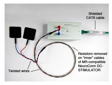
**Figure 6.2:** A shielded CAT6 cable and twisted "inner" cables were used to minimise current-induced magnetic fields while delivering current to the scalp electrodes. The stimulator device was placed outside the MSR.
