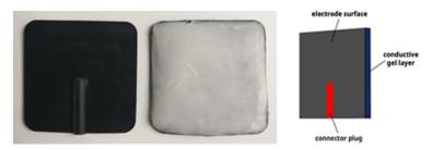
**Figure 5.4:** *Left:* Silicone-rubber electrodes (5 x 5 cm) prepared for electrical stimulation with a thin layer of conductive paste. *Right:* Corresponding electrode definition, including connector plug, specified in SimNIBS for FEM of induced electrical fields.
