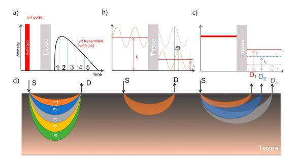
**Figure 1.13:** Schematic of the three NIRS techniques. (a) Time-domain NIRS; (b) Frequency-domain NIRS; (c) Continuous-wave NIRS; (d) Illustration of the resulting net photon path; reproduced from Lange and Tachtsidis, 2019.
