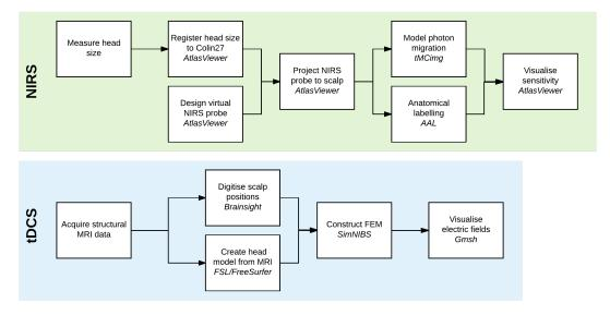
**Figure 5.1:** Schematic illustration of pipeline for the modelling of tDCS electrode and NIRS optode configurations.
