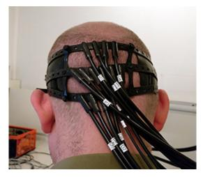
**Figure 5.2:** Combined optode-electrode montage for tDCS-NIRS of the visual cortex. The NIRS array is centred over EEG position Oz and held in place by three rubber head bands (spaced approximately 30 mm apart). tDCS electrodes are centred over PO7 and PO8 and attached to the head with a layer of ten20 conductive paste.
