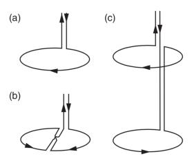
**Figure 1.11:** Flux transformer geometries for MEG. (a) magnetometer; (b) planar gradiometer; (c) axial gradiometer; reproduced from Hansen et al., 2010.
